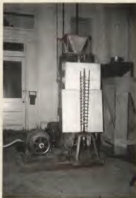
Fig. 2. Hydraulic grinding mill without the casing.
