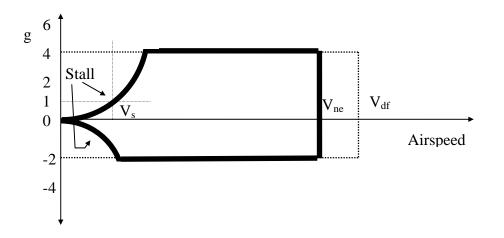
This is nearly the full flight envelope, and the airplane can be flown anywhere within the dark box on the g-Airspeed (often called V-N) diagram quite safely. However because the designer's a clever chap and can not only do maths, but understands aerodynamics as well, there are a couple of extra tricks to get through before finishing.
