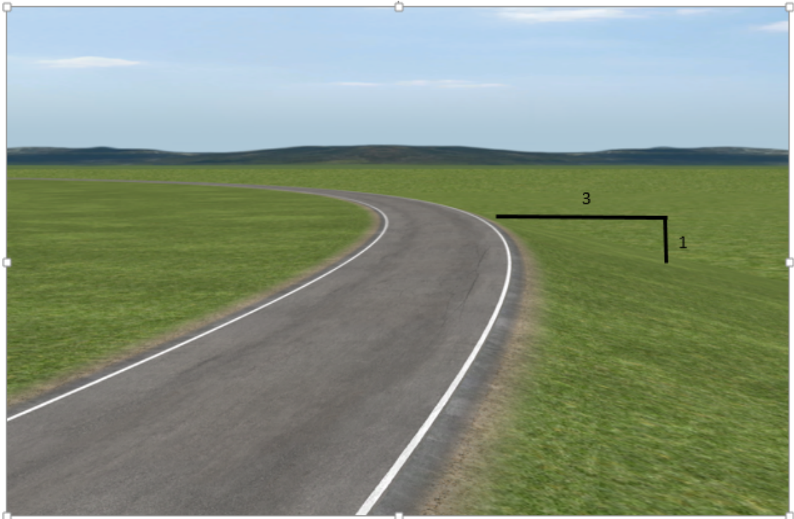
Figure 6 621.79 meter radius road with a 3:1 side-slope
