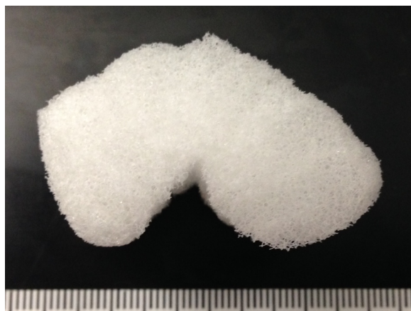
Figure 7: Image of 250um step foam that was unsuccessfully processed. This was the first result of my thesis. From this, there is an established upper limit for the amount of reticulation possible by means of the current foam processing method.
