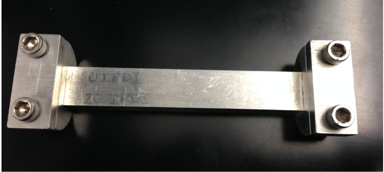
Figure 4: Volume actuation stability plate. The plate used to hold the foams upon the wire used to perform SMP foam actuation experiments.
