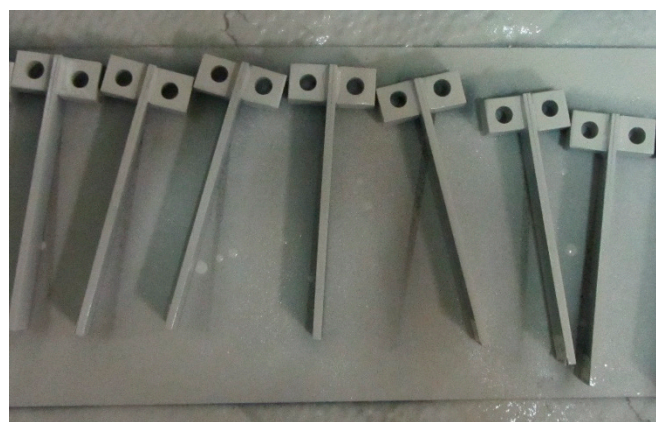
Figure 3. Double cantilever beam (DCB) samples after white painting.
