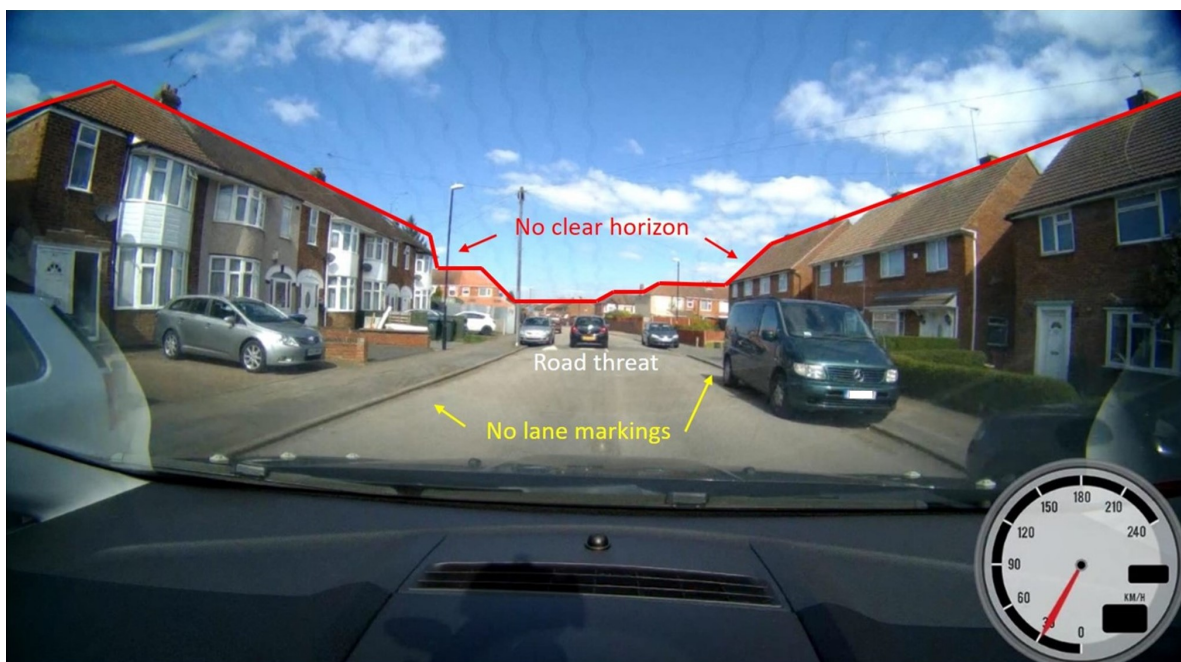
Figure 13. Corner case driving scenario including unclear horizon line, non-existing lane markings and obstructed road bump obstacle.
