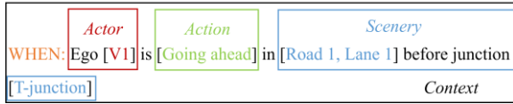
Fig. 1. SDL standard format example, which includes actors, actions, scenery and the overall context
