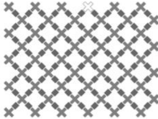
Figure 1. Connection-scheme of a 53 (working)-qubit Sycamore processor (adapted from Arute et al. 2019a, 505). Solid crosses denote qubits that work; outlined crosses denote qubits that don't work. "Squares" represent "adjustable couplers".
