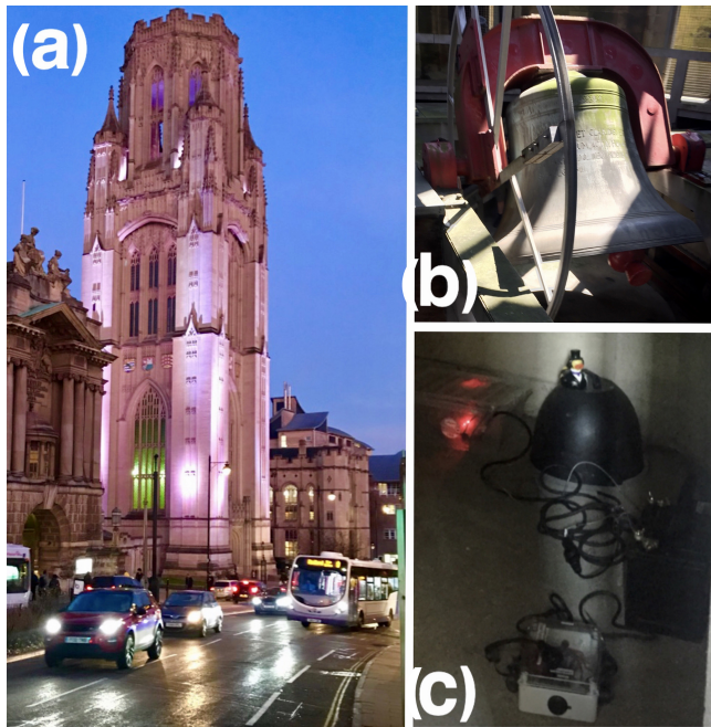
Figure 1. Great George bell (b) sits within the belfry of the Wills Memorial Building pictured in panel (a) on a typical weeknight. The broadband seismometer (c) installation set up in one of the alcoves above the bell. The instrument itself lies beneath the black dome with the Brunel rubber duck (geophysics group mascot) on top.
