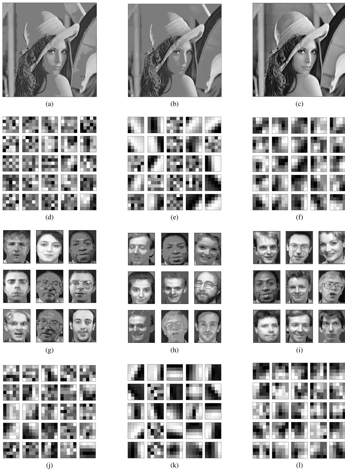
Fig. 5. Reconstructions of image Lena (top row) using the algorithms (a) IHT, (b) IST and (c) ICT and the filters learned using (a) IHT, (b) IST and (c) ICT.
