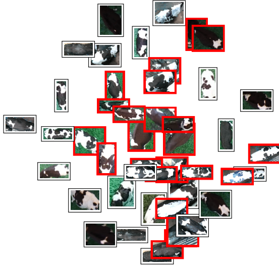
Figure 14: Class Examples Overlay. A randomly chosen example from each class overlaid on the centroids of the embeddings for their respective training instances, where half of the classes (highlighted in red) were not shown during training. Dimensionality reduction from n = 128 to 2 was performed using t-SNE [95] and the embedding was trained using Softmax and reciprocal triplet loss.
