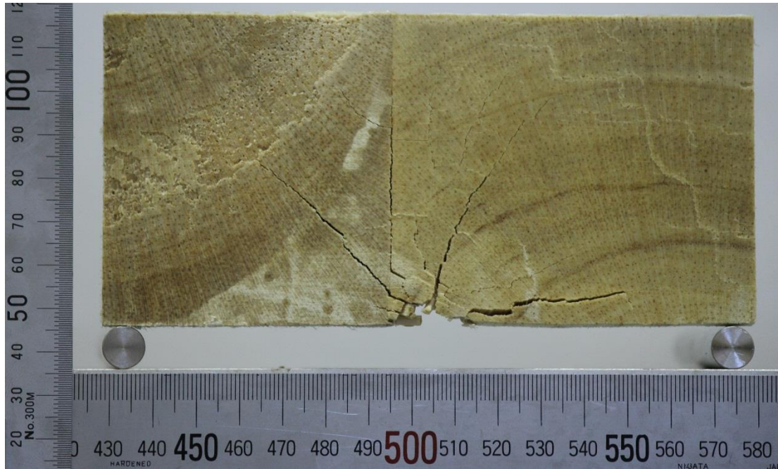
Fig. 15. Radial crack propagation from the impact point to the vicinity of Balsa HD core subjected to 120 J impact.
