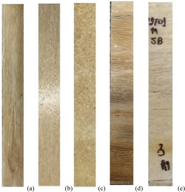
Fig. 4. Samples with longitudinally-oriented fibre layers: (a) alternating holes, (b) no holes; (c) randomly oriented ground fibres; samples with transversely oriented fibre layers: (d) alternating holes, (e) no holes.
