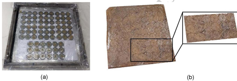
Figure 2. Coir fibre laminate manufacturing process: covered mould with undulations (a), and manufactured plates with resulting skin (b).
