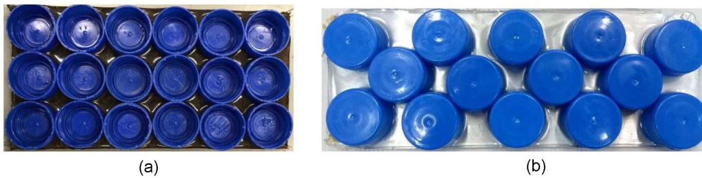
Figure 1. Bottle caps placed in cubic (a) and orthotropic (b) cell packing system.
