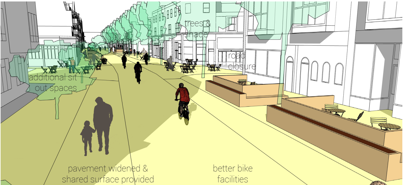
fig. 10 View of Palmerston Rd LTZ showing pavement widening, bike lane, planting, and additional facilities for external seating for existing commercial premises.
