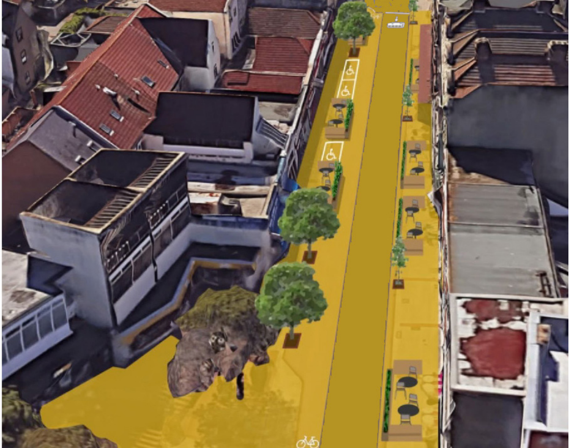
fig. 9 Ariel view of Palmerston Rd LTZ showing pavement widening, bike lane, planting, disabled parking, and additional facilities for external seating for existing commercial premises.
