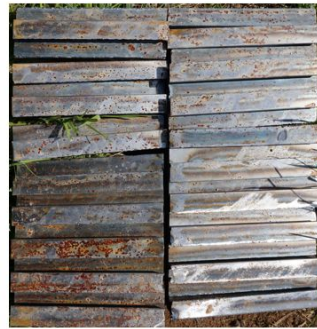
Auxetic core, post-explosion. The welding were broken and the auxetic did not perform an effective negative Poisson's ratio to absorb the impact energy.
