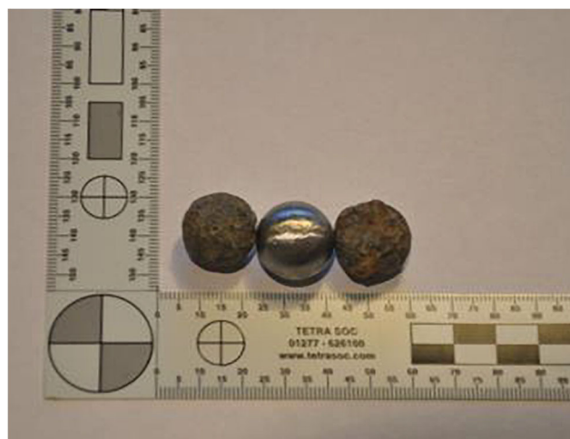
Fig. 1 Modern cast test projectile between two historical examples recovered from the Thames Foreshore
