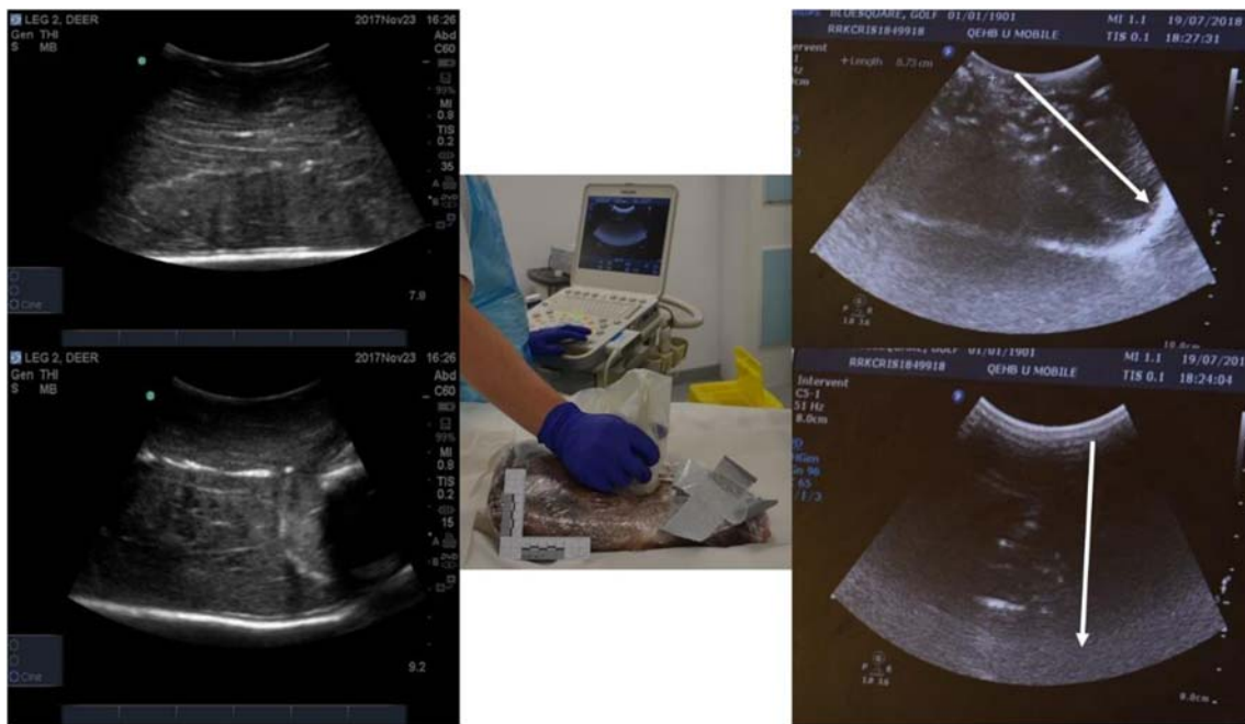
Fig. 4 Left, top, and bottom—pre-contrast, pre-shoot ultrasound images; centre—ultrasound in progress, demonstrating curvilinear probe compression of limb soft tissue; right, top, and bottom—post contrast injection ultrasound, highlighted areas represent GSW track, arrows indicate projectile direction of travel
