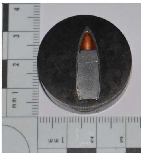
Fig. 2 Mounted section of 7.62-mm projectile. Mean core hardness 7.8Hv (SD 0.6Hv, n=3 ), lead mixed with antimony. Mean jacket hardness of 184.4Hv (SD 12.3Hv, n=3 ), steel with internal and external copper washes [12]
