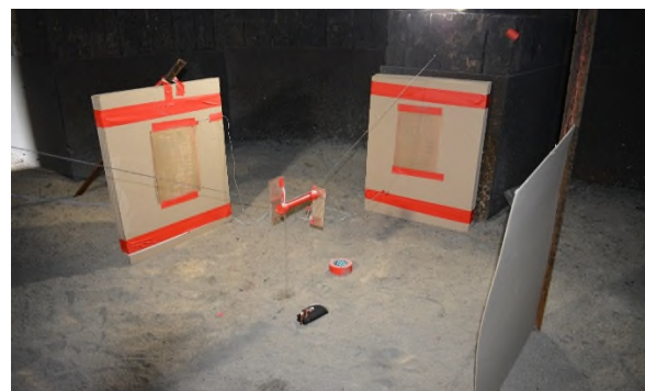
Figure 4 – Experimental set up for capturing fragments and record their velocities.
