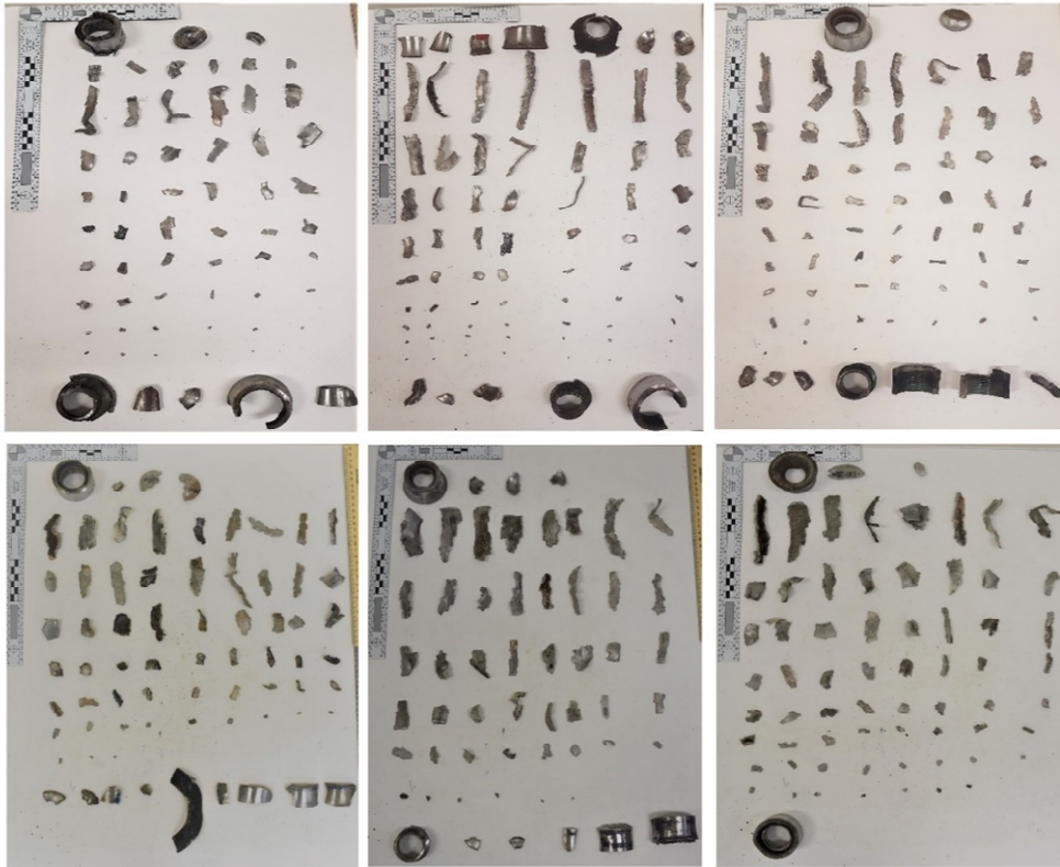
Figure 5 - Fragments of seamless steel pipes filled with Aluminized Ammonium Nitrate categorized as bottom end cap (top line), pipe body (middle) and top end cap (bottom line), where the detonation took place. Three samples (pipe #1, #2 and #3) of 38 mm diameter x 229 mm length (top) and three samples (pipe #4, #5 and #6) of 34 mm diameter x 229 mm length (bottom).
