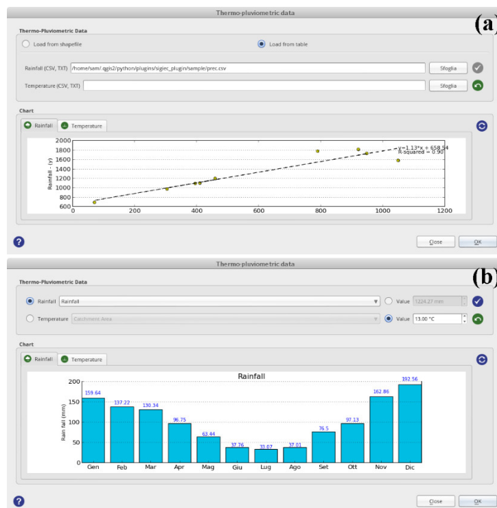
Figure 4. Graphical User Interface of stage 3. (a) Linear regression obtained after the input of the thermo-pluviometric data as a table. (b) Histogram plot showed by the plug-in if the user loads the data as a point vector layer.
