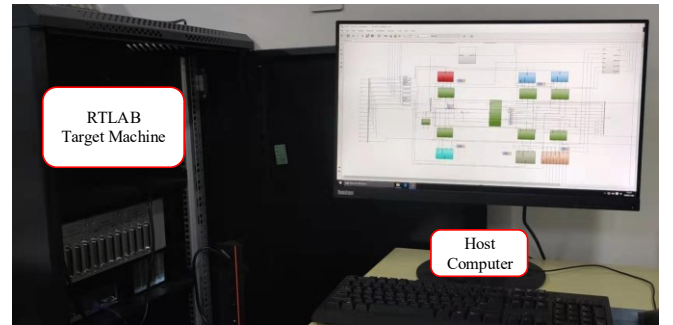
Fig. 6. Real-time simulation platform based on RT-LAB
