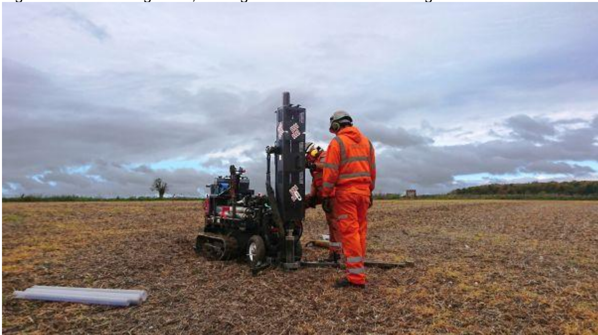
Figure 12: Dando Terrier rig in action at 5A looking north-west to anomalies 6A–7A, Strangways and Larkhill
