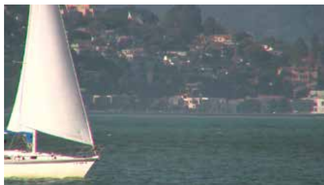
Image from a surveillance camera at sea. Chromatic aberration causes colored fringes around the edges of the boat's sail.
