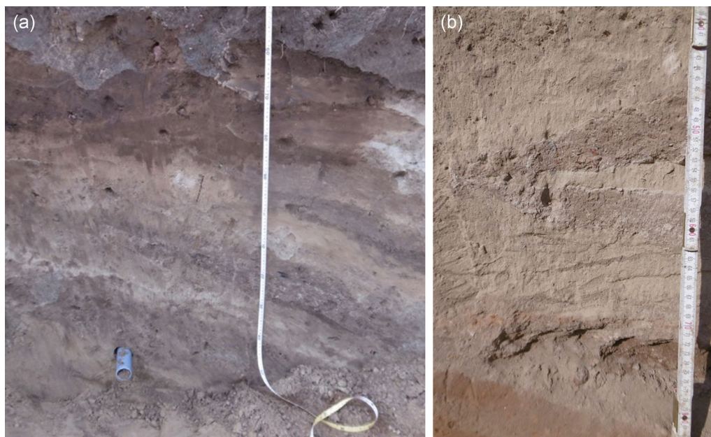
FIGURE 7 (a) Inclined dump of irregularly alternating sands with varying carbonate content, area A; (b) irregularly alternating calcareous sands in area B—wall opposite pit (see 6b) [Color figure can be viewed at wileyonlinelibrary.com ]
