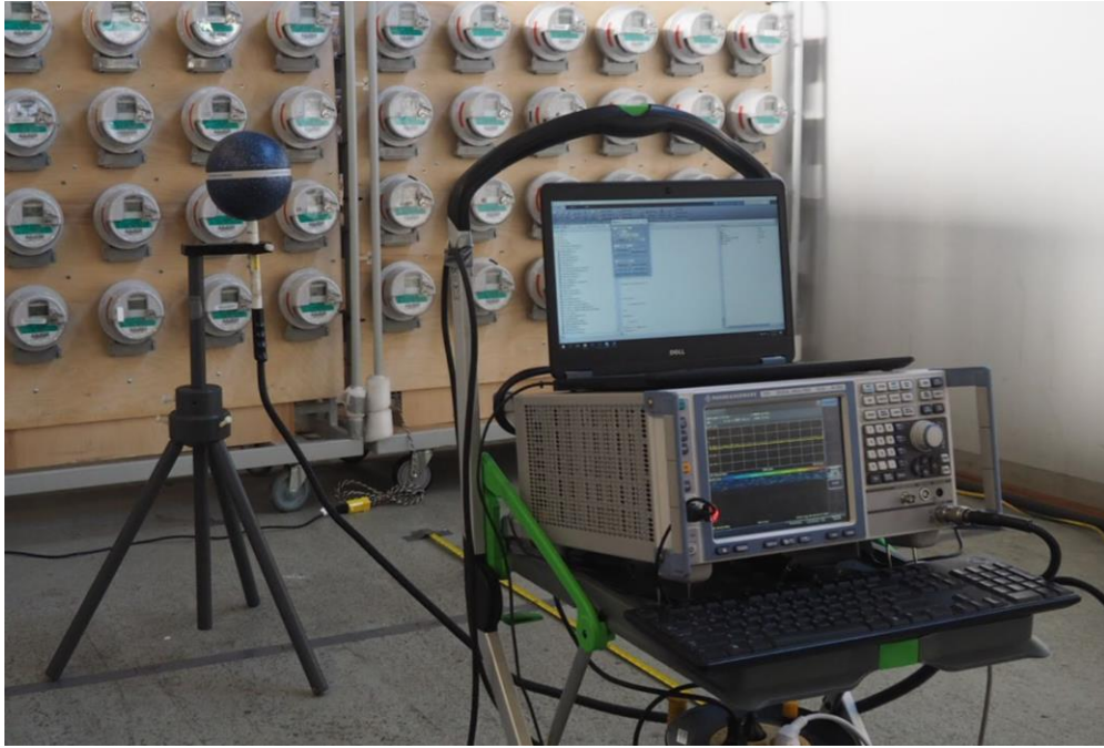
Figure 2: Measurement setup consisting of a Rohde & Schwarz FSV30 signal and spectrum analyzer (SA), connected to a laptop with Matlab software, combined with an R&S TS-EMF-B1 isotropic tri-axial antenna.
