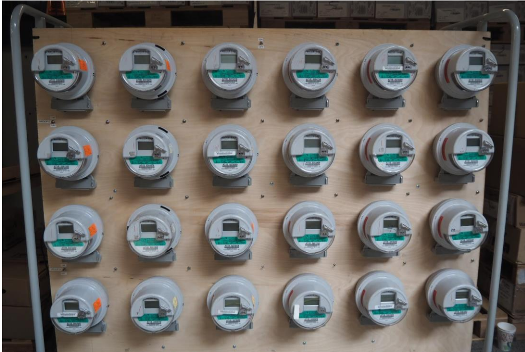
Figure 1: 24 AMI meters (type Aclara I-210+cn, NIC-511) attached to hardwood panel and mounted on a movable cart for easy configuration. Each row, column, or individual meter could be powered on/off.
