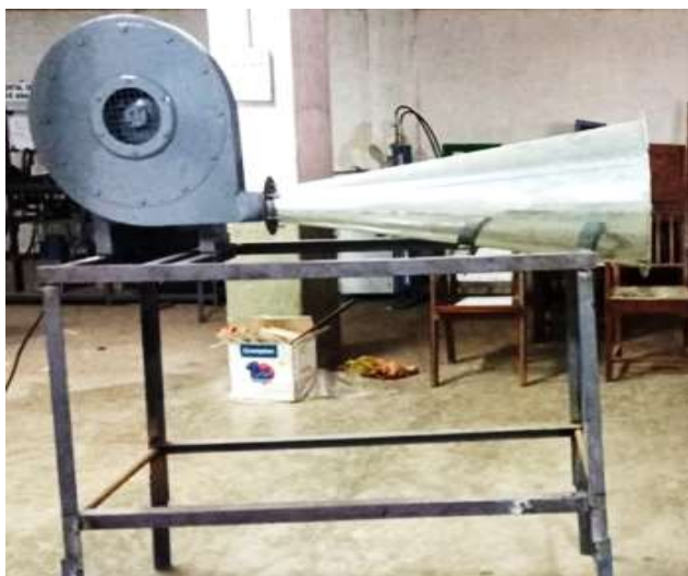
Fig. 5. Three coil cavity receiver wind test setup.
