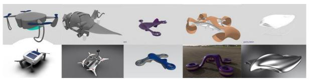
Figure 12. VR sketches created during the design process (top row) and the final render of the same product (bottom row)
