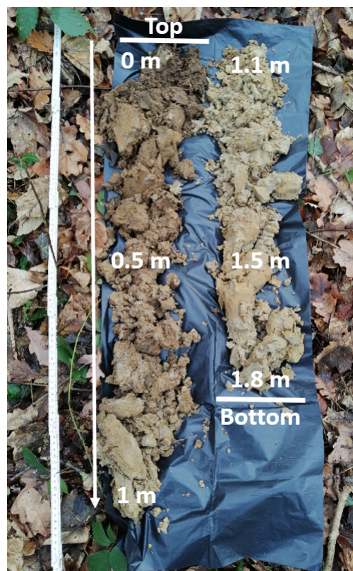
Figure 6. Output from auger drilling arranged according to approximate depth in the subsurface.
