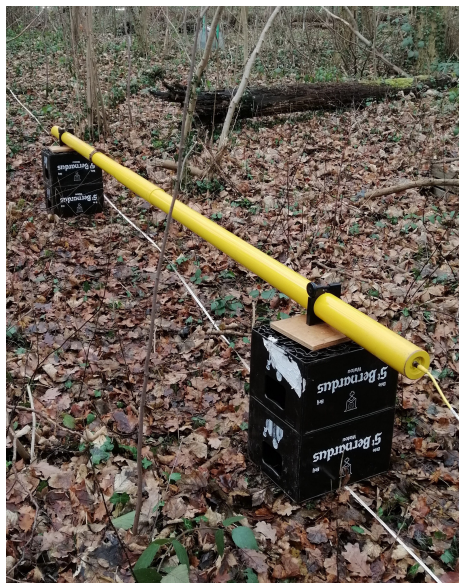
Figure 5. Multi-receiver FDEM measurement using a multi-receiver instrument at 0.6 m height; transmitter and receiver coils are arranged as sketched in Figure 1 with an additional HCP/PRP coil pair at 4 m/4.1 m, respectively.
