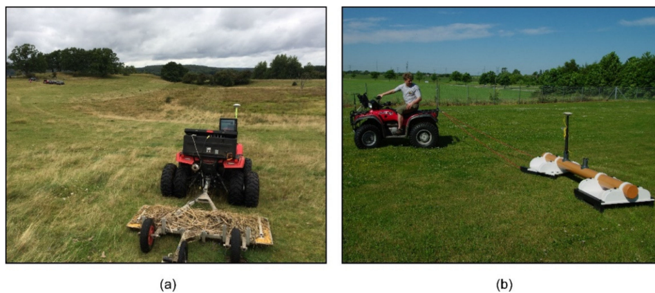
Figure 3. Survey configuration of: (a) the three-dimensional ground penetrating radar (3D-GPR) instrument and (b) the DUALEM-21S sensor.
