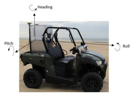
Figure 24: Mounting angle errors of the mobile LiDAR system.
