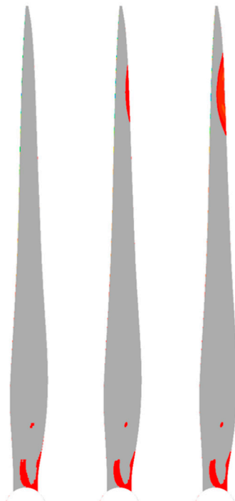
Figure 9. Zero net flow rate gusts separation region (in red) over the blade suction side at 90° azimuth angle: (left) unguasted case, (center) case with A_g = 5 m/s, and (right) case with A_g = 10 m/s.
