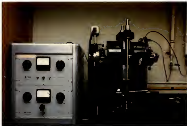
Fig. 3.1.3 Carver hydraulic laboratory press in an electromagnet. This system was used for aligning the powder in a magnetic field during pressing.
