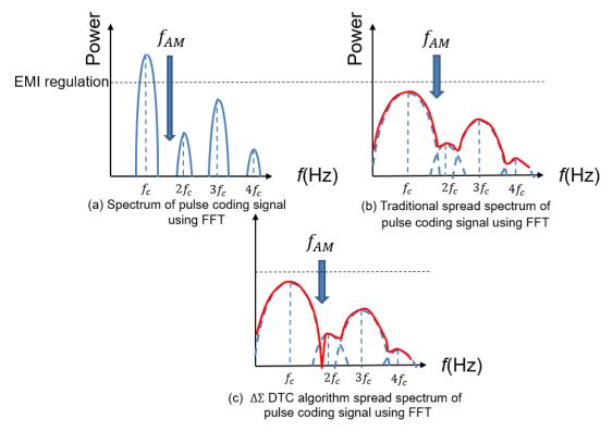
Figure 1.2 Spectrum of pulse coding signal.
