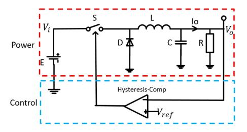
Figure 2.24 Basic hysteretic control buck converter.
