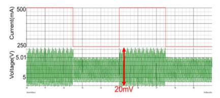
Figure 4.17 Transient response characteristics of PWPC method.
