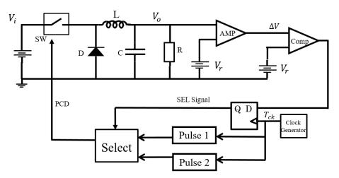
Figure 4.1 Switching converter with pulse coding.
