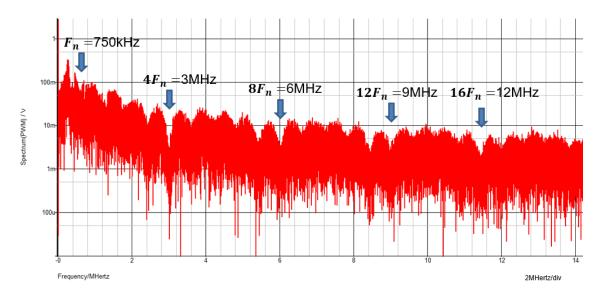
Figure 5.20 Simulated spectrum with EMI reduction using PWPC method.
