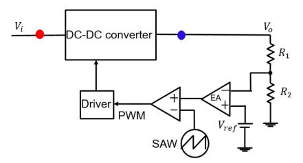
Figure 2.2 Basic configuration of DC-DC switching converter.
