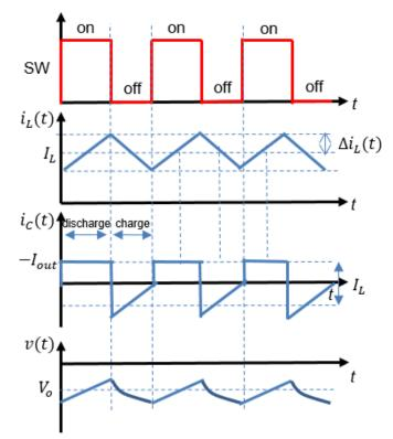
Figure 2.23 Timing chart of the buck-boost converter.
