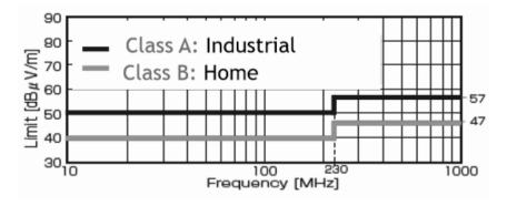
Figure 3.2 EMI regulation in radiation noise (CISPR22) in Japan.
