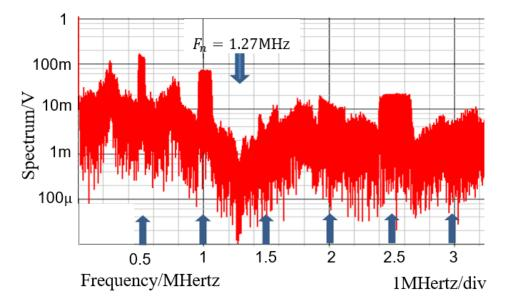
Figure 5.9 Simulated spectrum with EMI reduction in P = 2 situation.
