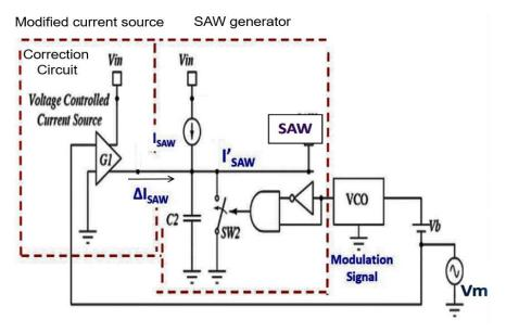
Figure 3.8 SAW generator & modified current source.
