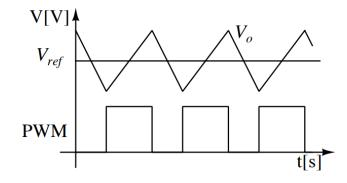
Figure 2.25 Operation waveforms of hysteretic control.
