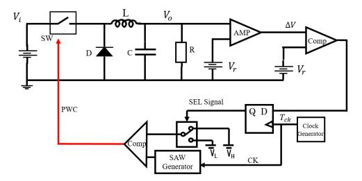
Figure 6.1 Converter with PWC control.
