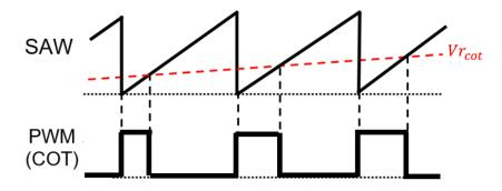
Figure 3.14 Timing chart of modified COT pulse. Fig. 3.15 shows the COT control method spectrum without EMI reduction, in which
