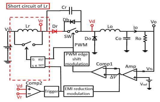
Figure 3.36 ZVS operation improvement circuit.
