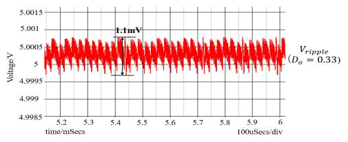
Figure 5.28 Output voltage ripple with full automatic notch frequency generation.
