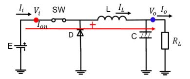
Figure 2.6 Buck converter when switch (SW) turns on.
