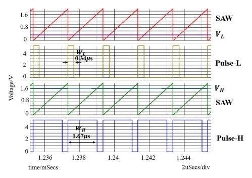
Figure 5.5 Simulation waveforms of Pulse-L and Pulse-H generation in P = 1 situation.
