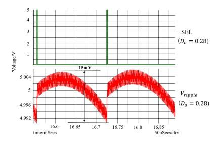
Figure 5.23 Waveforms of the select signal and ripple of output voltage in D=0.28 situation.
