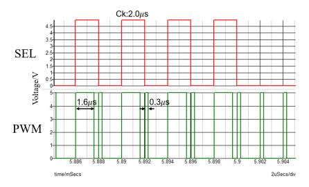
Figure 4.4 Main signal waveforms of PWC method.
