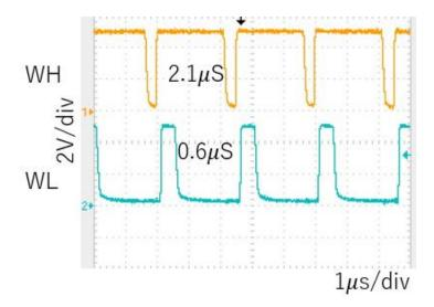
Figure 6.14 Experimental waveforms of  $W_H$  and  $W_L$  ( $F_{in} = 600 kHz$ ).
