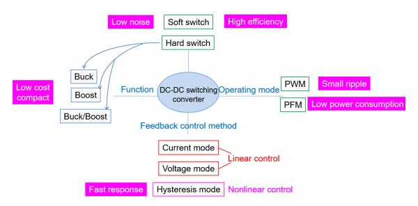
Figure 2.1 Performance of DC-DC switching converter.
