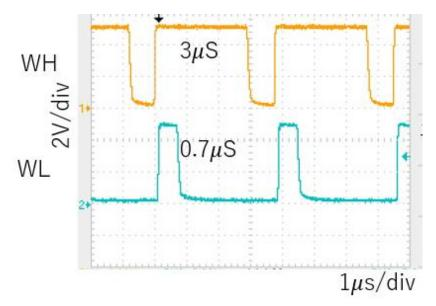
Figure 6.10 Experimental waveforms of  $W_H$  and  $W_L$  ( $F_{in} = 400 kHz$ ).
