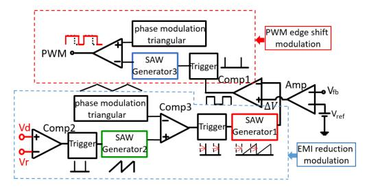
Figure 3.33 Circuit of the output ripple cancellation method.
