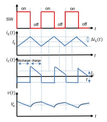
Figure 2.19 Timing chart of the boost converter (CCM).
