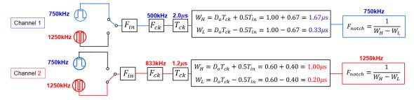
Figure 5.12 Block of change channel 1 to channel 2.
