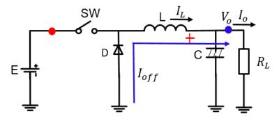
Figure 2.7 Buck converter when switch (SW) turns off.
