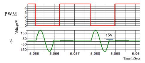
Figure 3.37 Waveforms of ZVS operation improvement.
