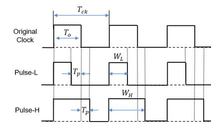
Figure 5.2 Timing chart of relationship between Pulse-H and Pulse-L of PWM signals.
