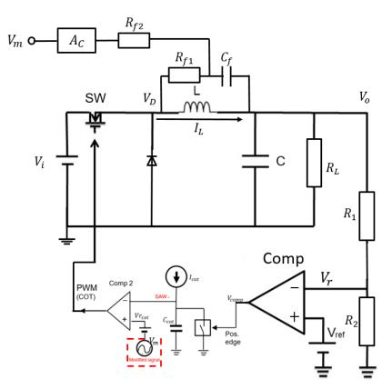
Figure 3.23 Circuit to cancel the output ripple.
