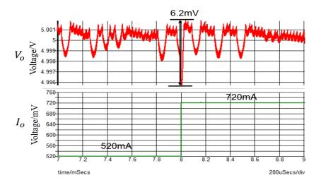
Figure 4.6 Transient response characteristics of PWC method.
