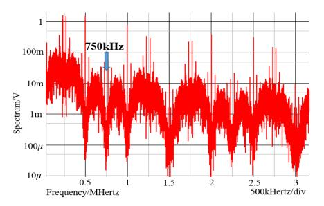
Figure 5.26 Simulated spectrum with full automatic notch frequency generation without EMI reduction.
