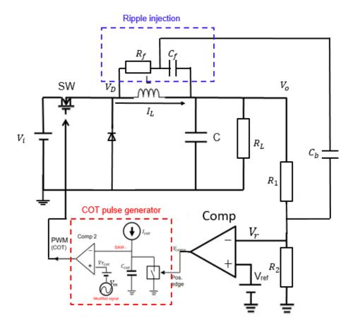
Figure 3.21 EMI noise reduction with the ripple injection method.
