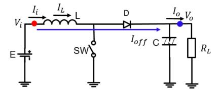
Figure 2.18 Boost converter when switch (SW) turns off.
