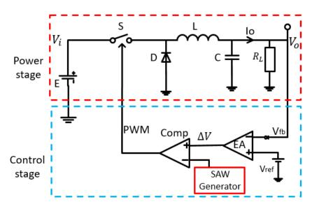
Figure 2.9 Voltage-mode negative feedback control circuit.
