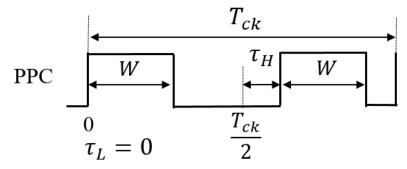
Figure 4.21 1 period 2 pulse trains of pulse phase coding signal.
