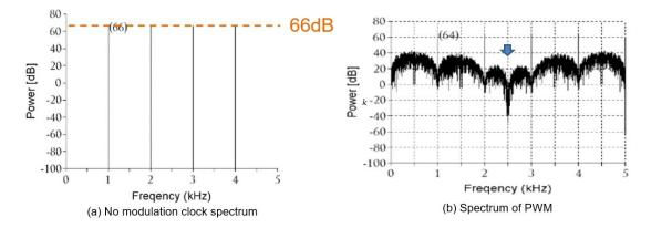
Figure 1.5 Spectrum of PWM using PWM  $\Delta\Sigma$  DTC.
