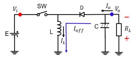
Figure 2.22 Buck-boost converter when switch (S) turns off.
