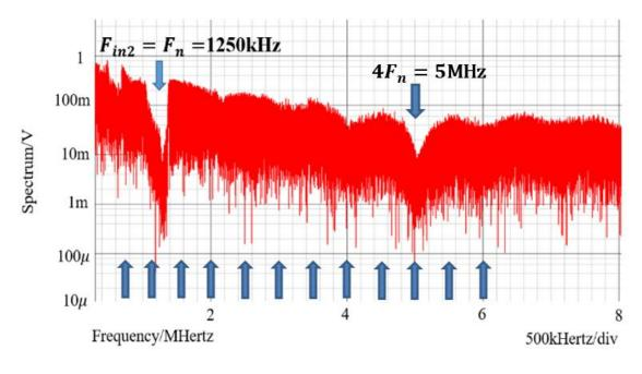
Figure 5.14  $F_{in2} = 1,250kHz$  situation.
