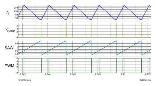
Figure 3.12 Waveforms of COT type hysteretic control converter.
