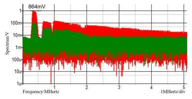
Figure 3.39 Spectrum of ZVS improvement circuit.
