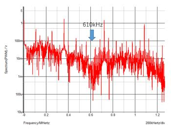
Figure 6.16 Simulation spectrum of PWM signal ( $F_{in} = 600 kHz$ ).
