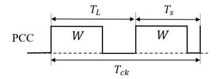
Figure 4.22 1 period 2 pulse trains of pulse cycle coding signal.
