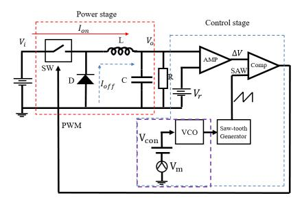
Figure 3.5 Frequency modulation of buck converter with PWM signal control.
