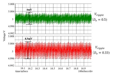
Figure 5.22 Change of the output voltage ripple.
