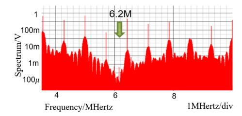
Figure 4.16 Spectrum of buck converter with PWPC control.
