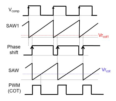
Figure 3.19 Block diagram of improved EMI noise reduction with the COT converter.
