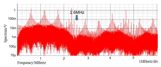
Figure 4.13 Spectrum of buck converter with PCC control (without EMI reduction).
