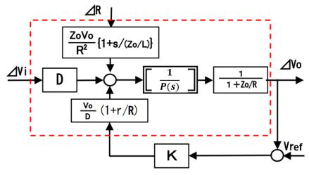
Figure 2.14 CCM block diagram of buck converter.
