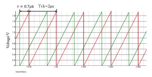
Figure 5.18 Waveforms of saw-tooth with period  $T_{ck}$  and delay  $T_{ck}$ .
