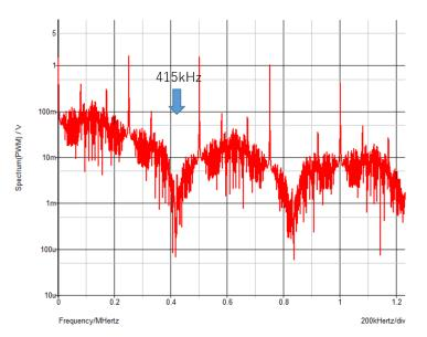
Figure 6.12 Simulation spectrum of PWM signal ( $F_{in} = 400kHz$ ).
