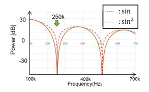
Figure 4.24 Comparison of notch characteristics with PWC method and PWPC method.
