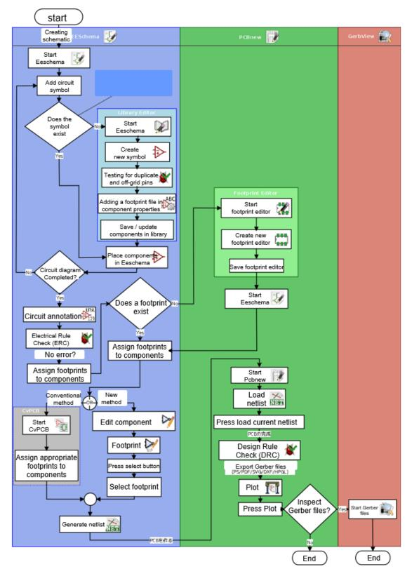
Figure 6.2 The flowchart for using Kicad software.
