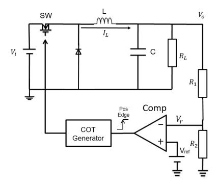
Figure 2.26 COT type hysteretic control buck converter.
