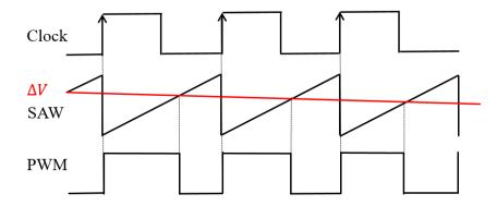
Figure 2.10 Waveforms in switching converter.
