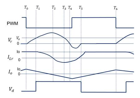
Figure 2.33 Timing chart of full-wave resonant soft-switching.
