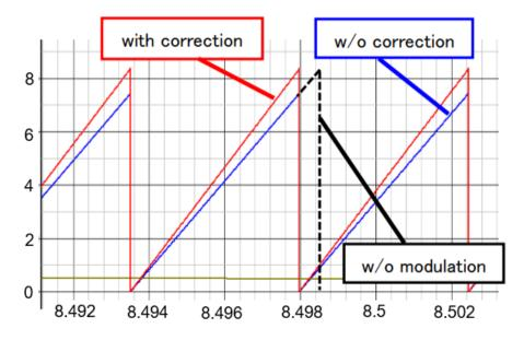
Figure 3.9 Comparison of SAW signals.
