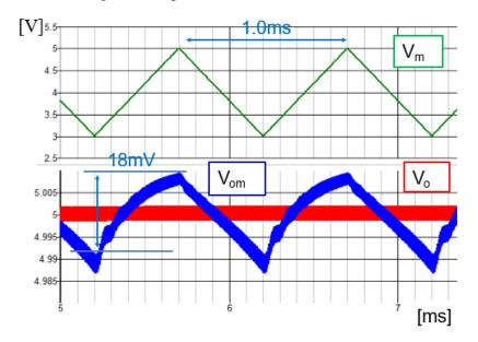
Figure 3.7 Output ripple with/without modulation.
