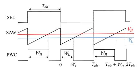
Figure 4.3 Main signal waveforms of PWC method.
