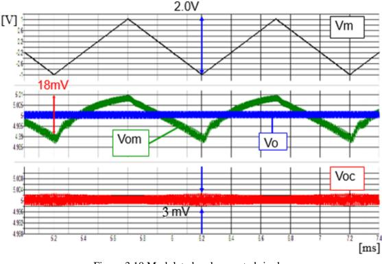
Figure 3.10 Modulated and corrected ripple.
