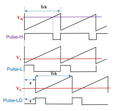
Figure 5.17 Timing chart of buck converter with PWPC control.
