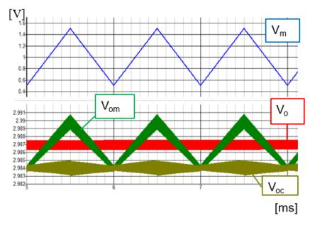
Figure 3.25 Cancellation of the ripple  $V_{oc}$ .
