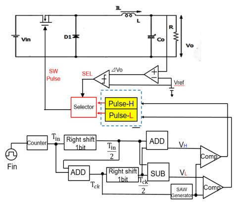
Figure 5.3 Pulse coding of automatic PWC method in P = 1 situation.
