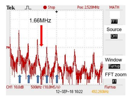
Figure 6.6 Spectrum of the PWC control switching converter.
