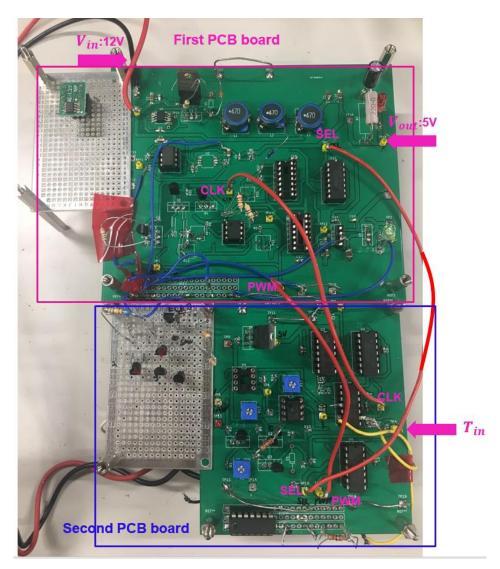
Figure 6.9 Automatic notch frequency generation PCB board circuit.
