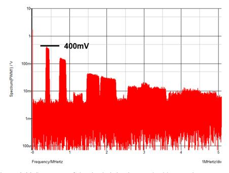
Figure 3.22 Spectrum of the ripple injection method hysteretic converter.
