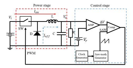
Figure 3.3 Buck converter with PWM signal control.
