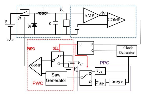
Figure 4.14 Buck converter with PWPC control.
