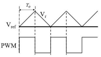
Figure 2.27 Timing chart of COT type hysteretic control buck converter.
