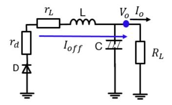
Figure 2.13 Off-period equivalent circuit.
