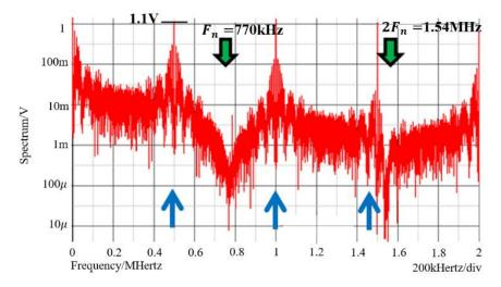
Figure 4.5 Spread spectrum with PWC control.
