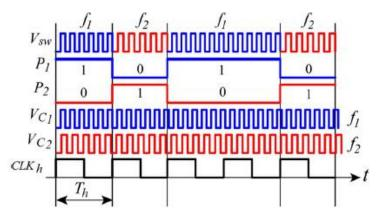
Figure 3.1 Waveforms analysis of a frequency-hopped buck converter with two hopping frequencies.
