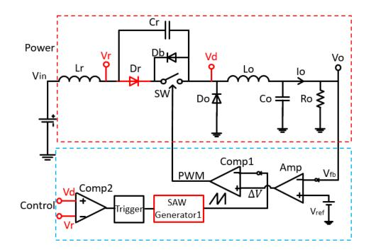
Figure 3.27 Circuit of the full-wave resonant converter.
