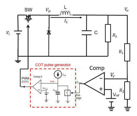
Figure 3.11 COT control method hysteretic control converter.
