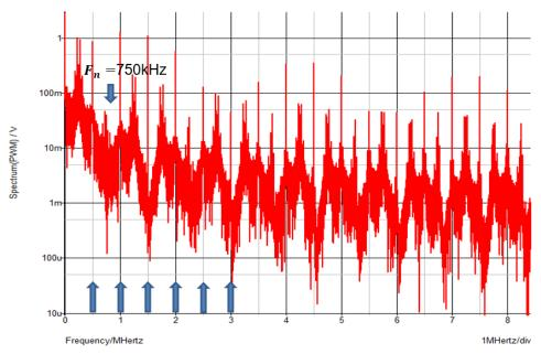
Figure 5.6 Simulated spectrum by PWM signal without EMI reduction when P = 1 situation.
