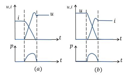
Figure 2.30 Voltage and current during hard switching (a): off-process (b): on-process.
