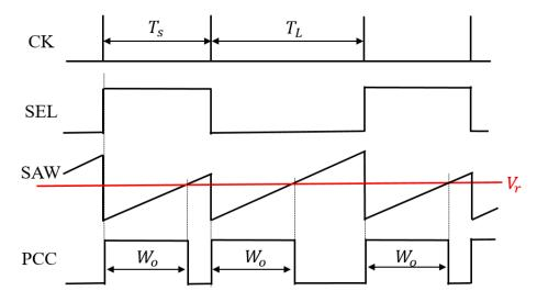
Figure 4.11 Main signal waveforms of PCC method.
