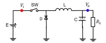
Figure 2.5 Basic circuit of buck converter.
