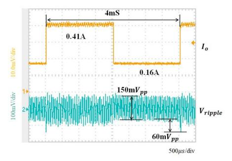
Figure 6.18 Transient response characteristics of the PWC method.
