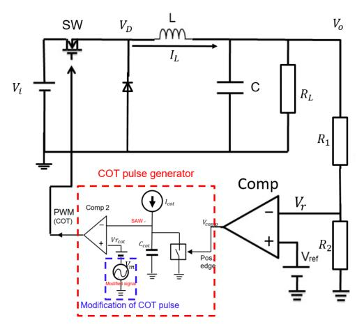
Figure 3.13 EMI noise reduction with COT control circuit.
