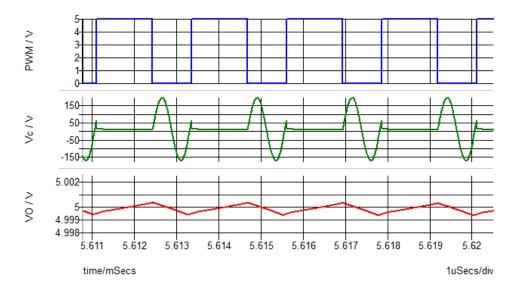
Figure 3.29 Simulation waveforms in EMI reduction modulation circuit.
