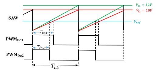
Figure 5.25 Main signal waveforms of *D* detection method.
