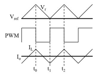
Figure 2.29 Waveforms of ripple injection converter.
