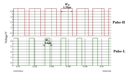
Figure 5.8 Simulation waveforms of pulse-H and pulse-L generation in P = 2 situation.
