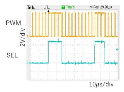
Figure 6.11 Experimental waveforms of PWM and SEL signals ( $F_{in} = 400 kHz$ ).
