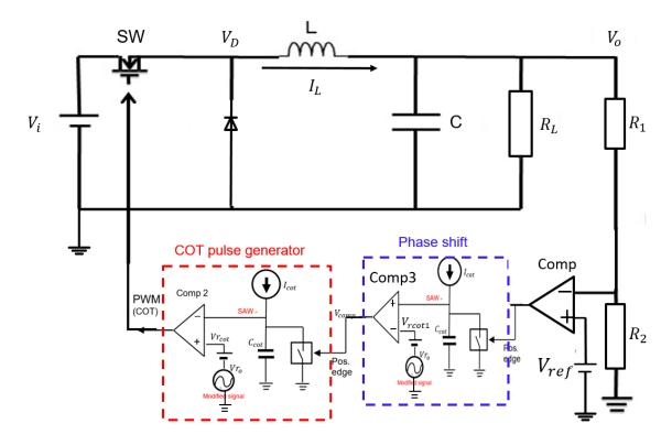
Figure 3.18 Improved EMI noise reduction with the COT control method.
