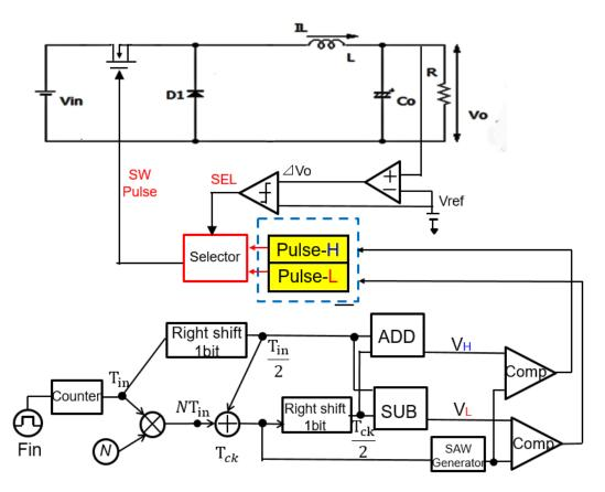
Figure 5.4 Pulse coding of automatic PWC method in P = N situation
