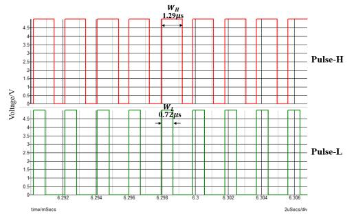
Figure 5.10 Simulation waveforms of Pulse-H and Pulse-L generation in P = 3 situation.
