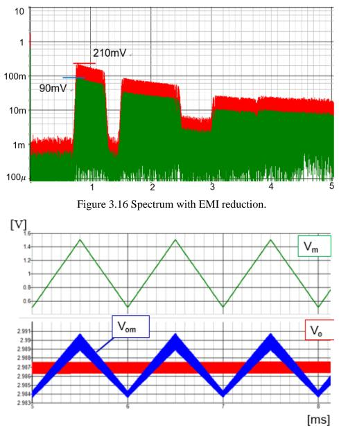
Figure 3.17 Output ripple with modulation.
