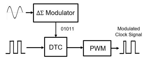
Figure 1.1Circuit structure of spread spectrum clock generator
