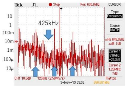
Figure 6.13 Experimental spectrum of PWM signal ( $F_{in} = 400 kHz$ ).
