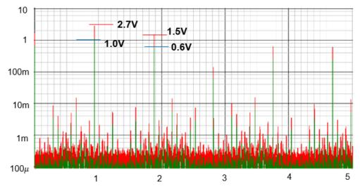
Figure 3.15 COT control method spectrum without EMI reduction.
