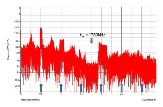
Figure 5.11 Simulated spectrum with EMI reduction in P = 3 situation.
