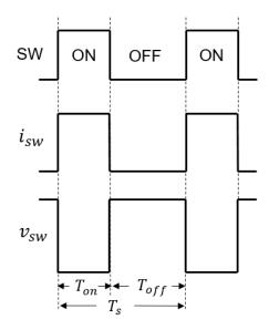
Figure 2.4 Switch state and switching waveform.
