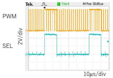
Figure 6.15 Experimental waveforms of PWM and SEL signals ( $F_{in} = 600 kHz$ ).
