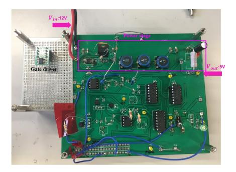
Figure 6.4 PWC control buck converter PCB board.
