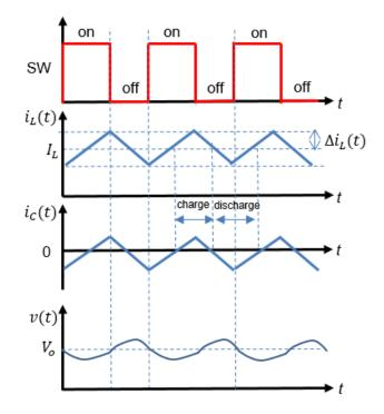
Figure 2.8 Timing chart of buck converter (continuous current mode (CCM)).
