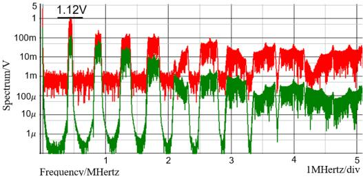
Figure 3.31 Spread spectrum of the soft-switching converter output.
