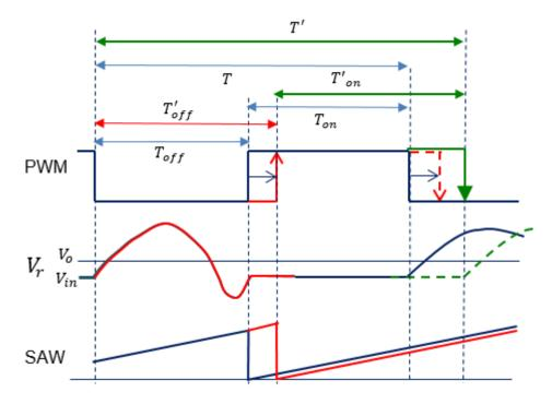
Figure 3.32 Waveforms in the ripple cancellation circuit.
