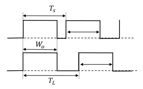
Figure 4.9 Coded pulses with the PCC method.
