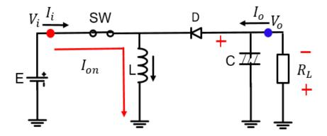
Figure 2.21 Buck-boost converter when switch (S) turns on.
