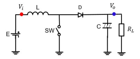
Figure 2.16 Basic circuit of the boost converter.
