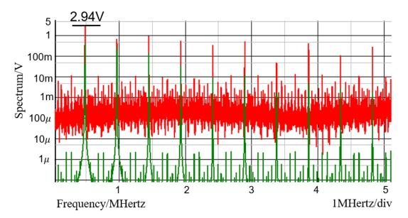
Figure 3.30 Spectrum of the soft-switching converter output.
