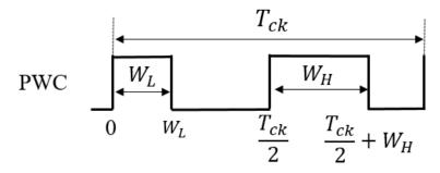
Figure 4.18 1 period 2 pulse trains of pulse width coding signal.
