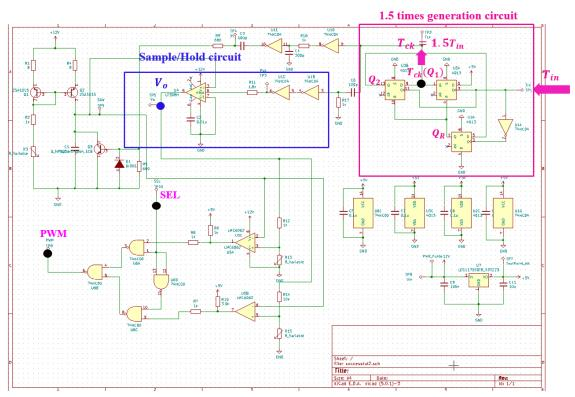
Figure 6.7 Automatic notch frequency generation circuit with Kicad.
