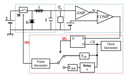
Figure 4.7 Buck converter with PPC control.
