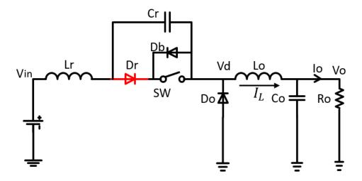
Figure 2.32 Full-wave resonant soft-switching.
