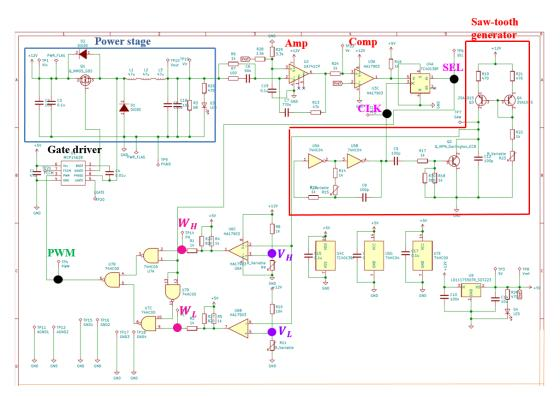
Figure 6.3 PWC control buck converter circuit with Kicad.
