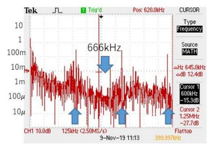
Figure 6.17 Experimental spectrum of PWM signal ( $F_{in} = 600 kHz$ ).
