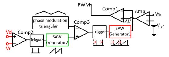
Figure 3.28 EMI reduction modulation circuit.
