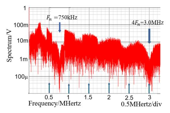
Figure 5.7 Simulated spectrum with EMI reduction in P = 1 situation.
