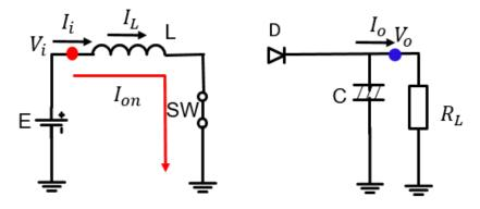
Figure 2.17 Boost converter when switch (SW) turns on.
