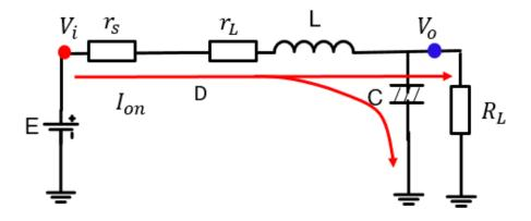
Figure 2.12 On-period equivalent circuit.
