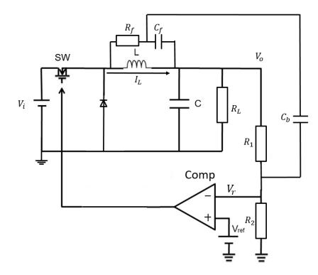
Figure 2.28 Ripple injection method buck converter.
