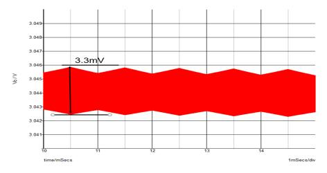
Figure 3.20 Output ripple with improved EMI noise reduction with the COT converter.
