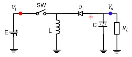
Figure 2.20 Basic circuit of the buck-boost converter.
