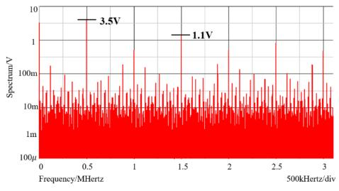
Figure 3.4 Simulated spectrum without EMI reduction.
