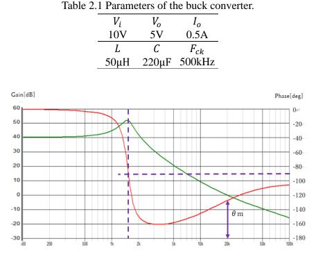
Figure 2.15 Bode diagram of the buck converter.
