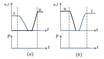
Figure 2.31 Voltage and current during soft switching (a): off-process (b): on-process.
