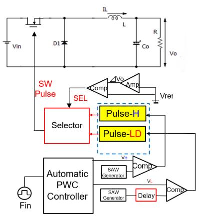
Figure 5.16 Pulse coding of PWPC method.
