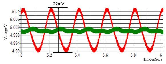
Figure 3.34 Output ripple with EMI reduction (red) and ripple cancellation (green).
