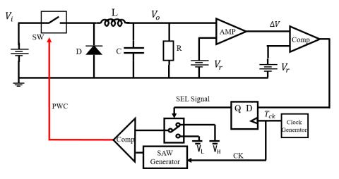
Figure 4.2 Buck converter with PWC control.
