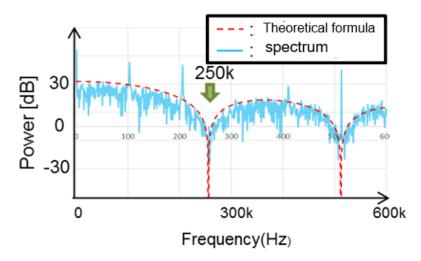
Figure 4.20 Comparison diagram between theoretical formula and spectrum.
