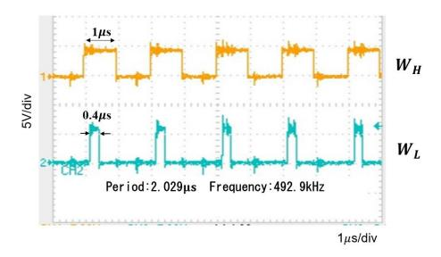
Figure 6.5 Waveforms of  $W_H$  and  $W_L$  in PWC control buck converter.
