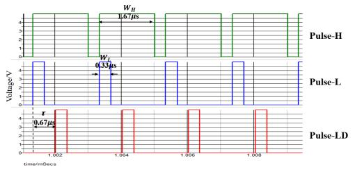
Figure 5.19 Main waveforms of PWPC method.
