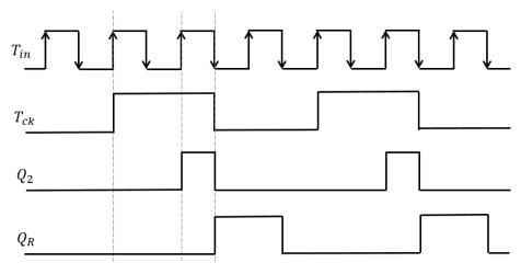
Figure 6.8 Main signal waveforms when using  $T_{in}$  create  $T_{ck}$ .
