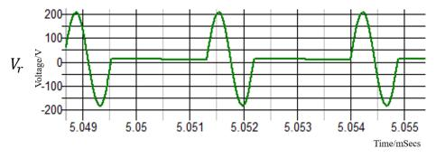
Figure 3.38 Simulation result of the resonant voltage improvement.
