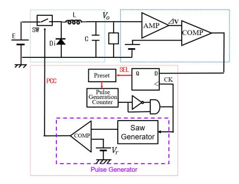
Figure 4.10 Buck converter with PCC control.
