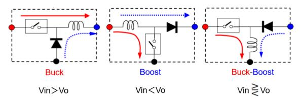
Figure 2.3 Basic constitution of buck, boost, and buck-boost converters.
