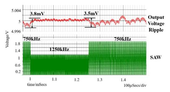
Figure 5.15 Automatic switching on transient response and saw-tooth.
