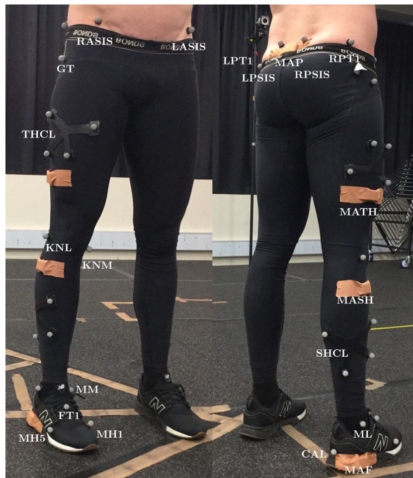
Figure 2. Optical motion capture (OMC) and magnetic, angular rate and gravity (MARG) sensor placement: CAL, calcaneus; FT1, foot tracking marker one; GT, greater trochanter; KNL, knee lateral; KNM, knee medial; LASIS, left anterior superior iliac spine; LPSIS, left posterior superior iliac spine; LPT1, left pelvis tracking marker one; MAF, foot MARG sensor; MAP, pelvis MARG sensor; MASH, shank MARG sensor; MATH, thigh MARG sensor; MH1, first metatarsal head; MH5, fifth metatarsal head; ML, lateral malleolus; MM, medial malleolus; RASIS, right anterior superior iliac spine; RPSIS, right posterior superior iliac spine; RPT1, right pelvis tracking marker one; SHCL, shank cluster; THCL, thigh cluster.
