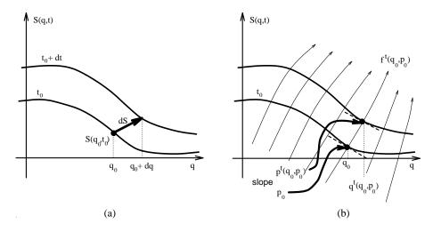
**Fig. 1.** (a) A wavefront S(q, t) plotted as a function of the position q for two different times. (b) The phase of the wavefront S(q, t) transported by a swarm of "particles"; Hamilton's equations (15) construct S(q, t) by transporting  $q_0 \rightarrow q(t)$  and  $p_0$ , the slope of  $S(q_0, t_0)$ , to  $p_0 \rightarrow p(t)$ .
