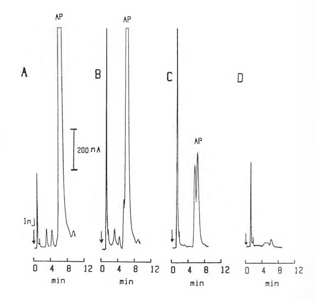
Fig. 3. (A). Recovery of AP from the DMSO-acid extraction medium (90% DMSO containing 0.12% metaphosphoric acid) at  $25^{\circ}$  with and without 0.05% AA in the medium. The initial concentration of AP in the medium was 1.5 mg/50 ml, and an aliquot of the DMSO-acid extract was diluted 5-fold with methanol prior to injection (0.02 ml) into the chromatograph. The standard error of the determination with 0.05% AA was  $\pm$  0.6%.
