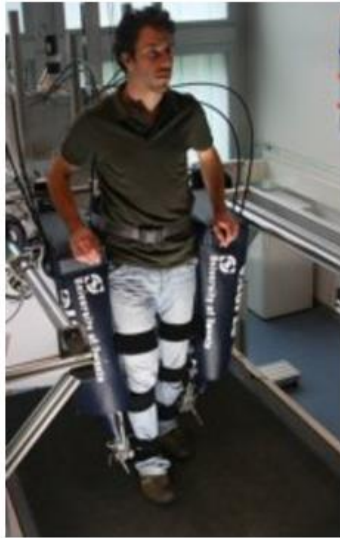
Subject's leg strapped to LOPES exoskeleton
