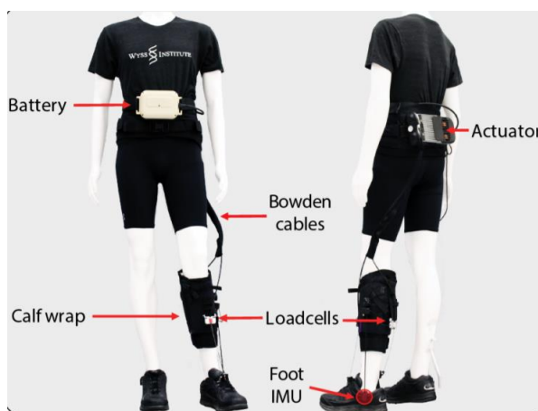
Fig. 1.22 A soft exosuit developed by Harvard University [1.64].
