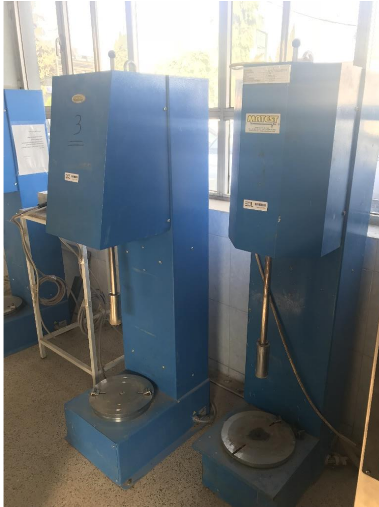
Figure 3.8 Compaction machine used in the study MATEST type.
