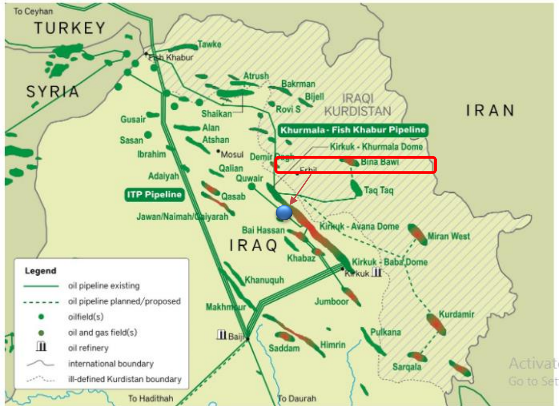
Figure 3.2 Iraq's oil and gas infrastructure (Butt, 2017).
