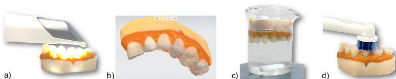
Fig. 1. Experiment workflow followed in the study. Scanning with IOS (a), obtaining the 3D model (b), immersion in the acid solution for simulated erosion (c), tooth brushing for simulated abrasion (d).
