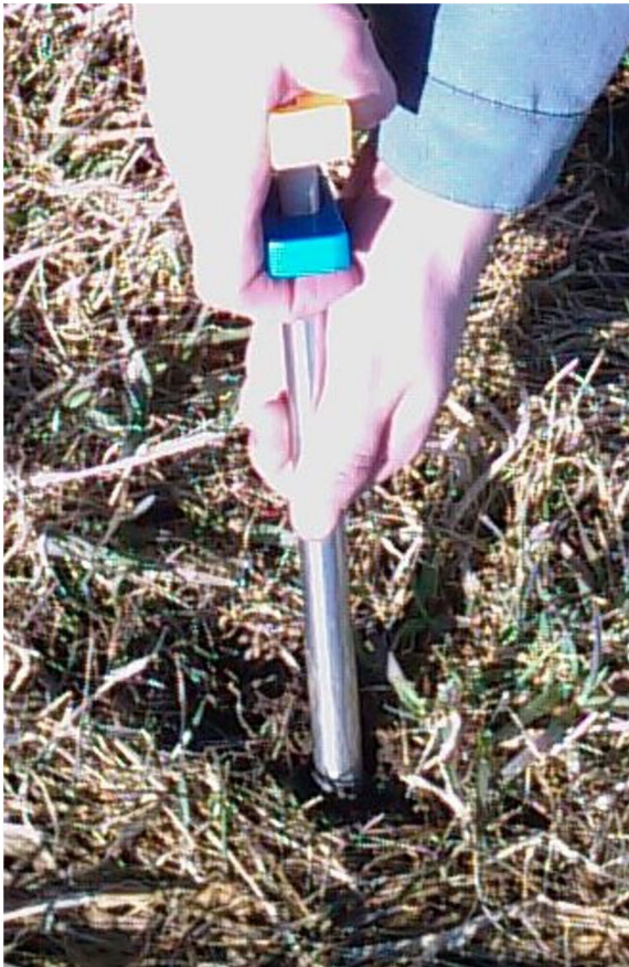
Fig. 1 Pasture soil sampling was performed with a cylindrical metal instrument, inserted in the ground to a depth of 3–4 cm. Photo was taken by Kristina Lindgren
