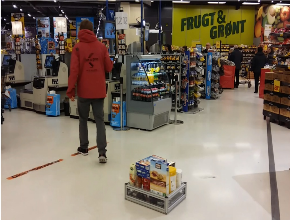
Figure 1 Test of an autonomous vehicle following a person in the Bilka-warehouse, Sønderborg, Denmark
