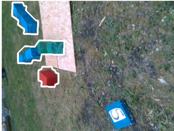
Figure 4.3: Example of YOLO neural network, that ignores object of correct color, but wrong shape (object with printed "5" on top)
