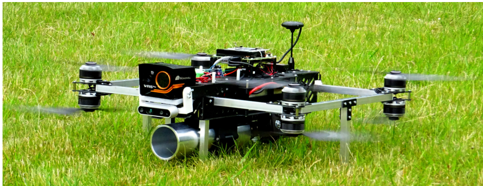
Figure 1.1: Photo of the designed, constructed, and tested UAV for the application in (semi)-autonomous fire-extinguishing scenarios.
