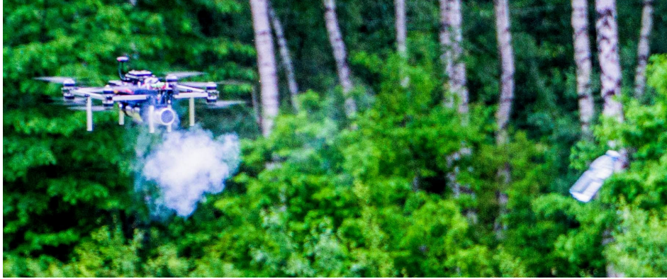
Figure 5.9: Fire extinguishing ampoule (replaced by water bottle in this experiment) discharged by the launcher.
