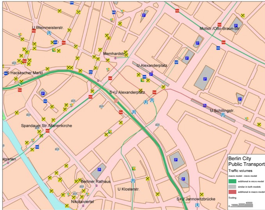
(a) Difference of micro and macro model in absolute values - A difference of less than 2000 trips per day is considered as similar in both models.
