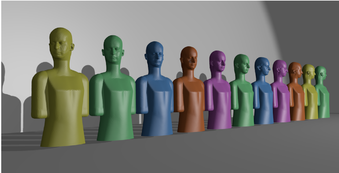
Figure 2: 3D surface meshes of FABIAN for numerical simulations up to 6 kHz, and head-above-torso orientations from -50^\circ (left) to 50^\circ (right).
