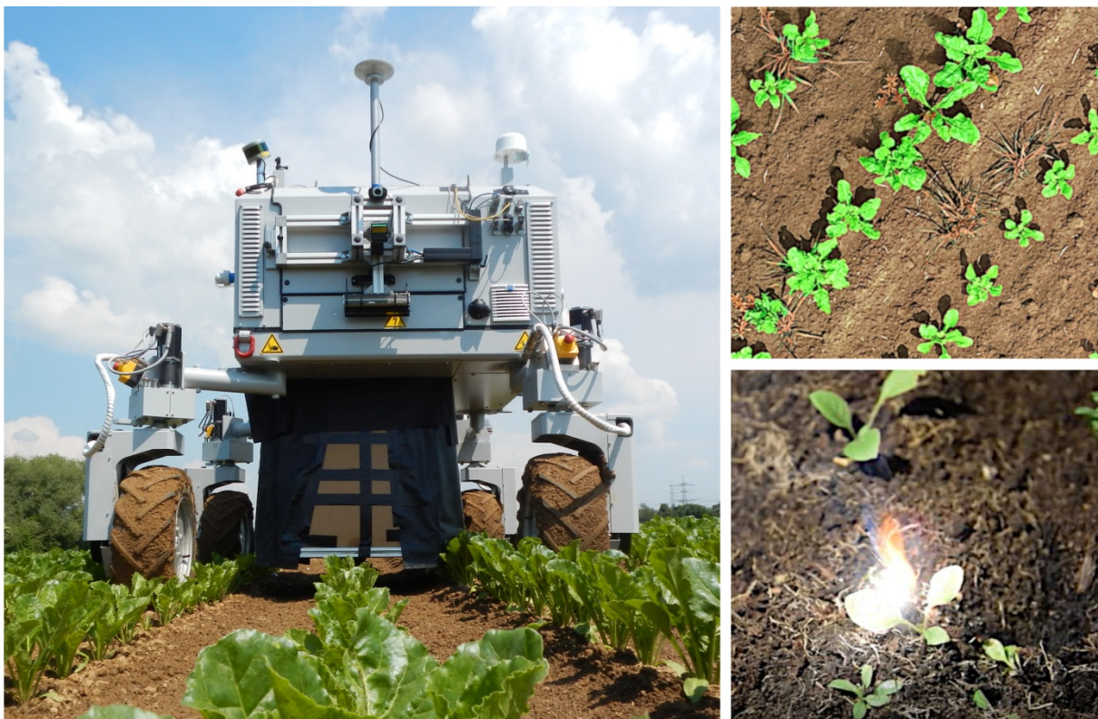
Fig. 6 Robot scanning an agricultural field with various sensors, classifying species, detecting weeds and targeting them for burning with a laser (left). Crop and weeds as seen from a robot (top right). Laser-burning a weed (bottom right). Pictures courtesy of CRC Phenorob, University of Bonn ( www.phenorob.de ).
