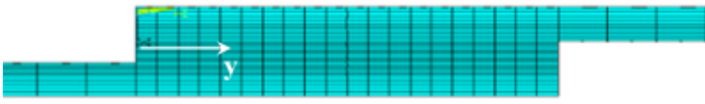
Figure 2.6 – Discretization of nodes and elements for Ansys APDL simulation.
