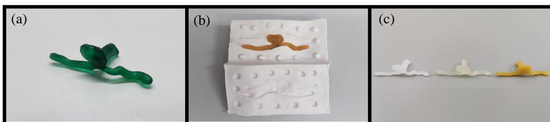
Figure 4.2 - Models obtained by rapid prototyping and lost wax. (a) model obtained by rapid prototyping of VisiJet FTX Green resin (microsla); (b) bipartite silicone mold; (c) paraffin sacrifice mold, glycerin-based soap and beeswax, respectively (full scale).
