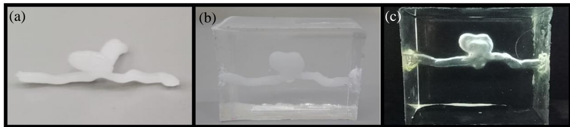
Figure 4.3 - Processing steps to obtain the final biomodel with paraffin. (a) Paraffin; (b) Biomodel after the cure of PDMS; (c) Final PDMS biomodel.
