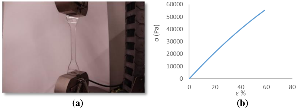
Figure 2.2 - (a) specimen positioned on the tensile machine. (b) PDMS stress-strain curve.
