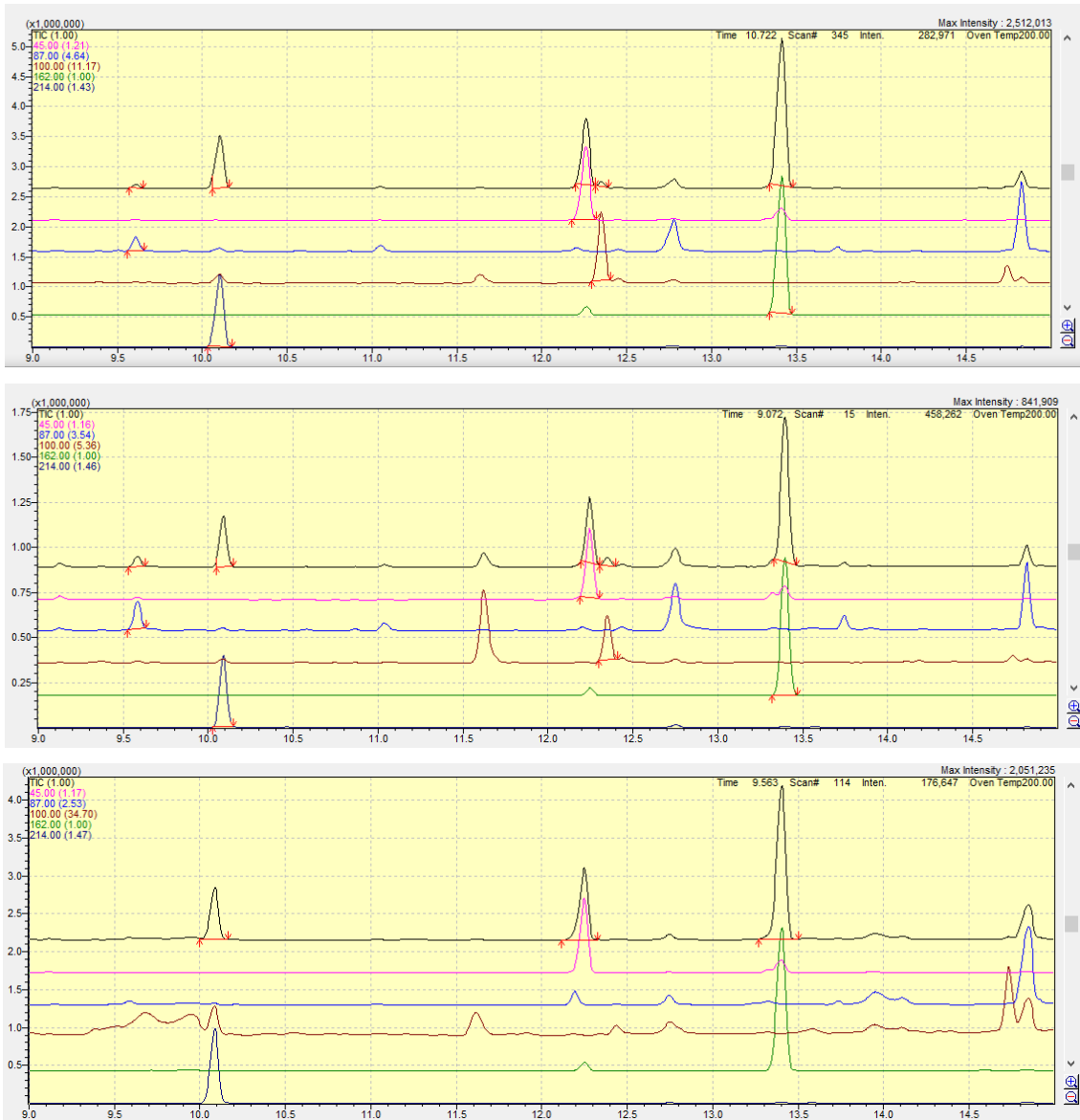
Figure 4.10. Comparison between the obtained chromatograms using SIM MS mode for SPME/GC-MS analysis of a standard mixture solution with 50, 10 and 1 µg/L concentration, from top to bottom.
