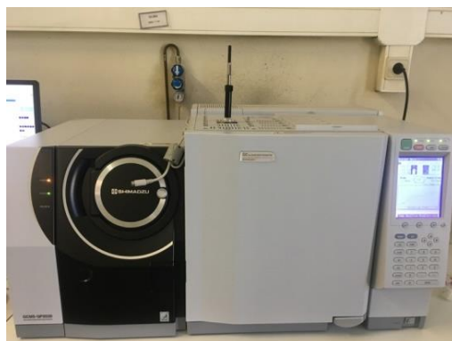
Figure 3.4. GC-MS with a SPME fiber inserted in the GC-MS injection port.
