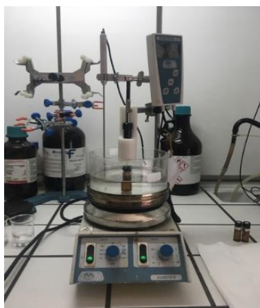
Figure 3.3. SPME extraction using a manual holder, an agitation and heating plate with temperature control and 4 mL amber vials.
