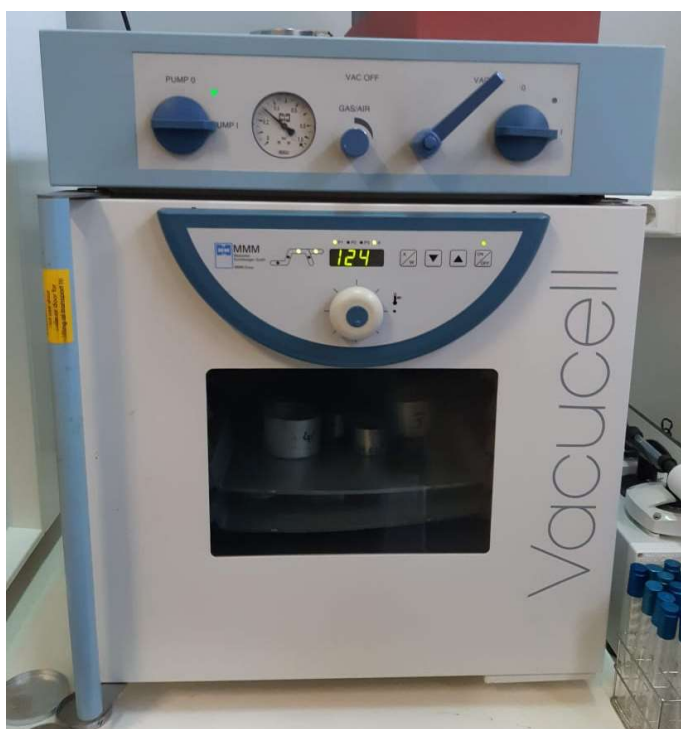
Figure 41: Samples on vacuum chamber before thermogravimetry tests.
