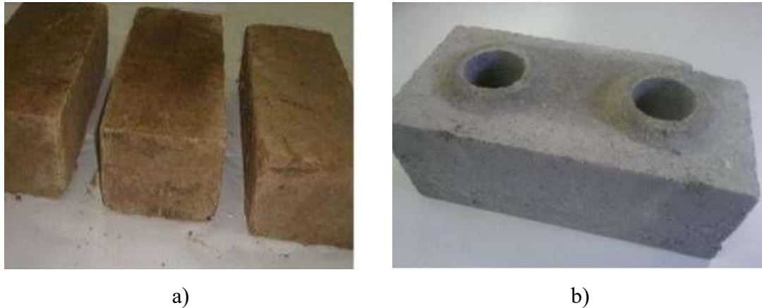
Figure 10: Different types of CEBs: a) Solid block [25] b) Interlocking block [26].
