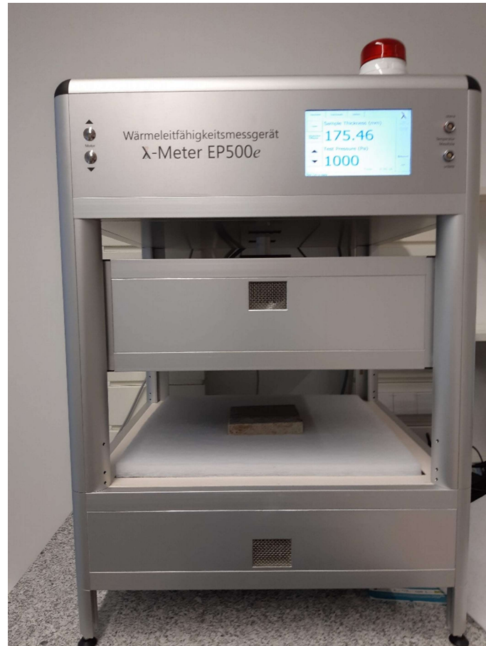
Figure 45: Lambda-Messtechnik® \lambda -Meter EP500e Guarded Hot Plate apparatus.
