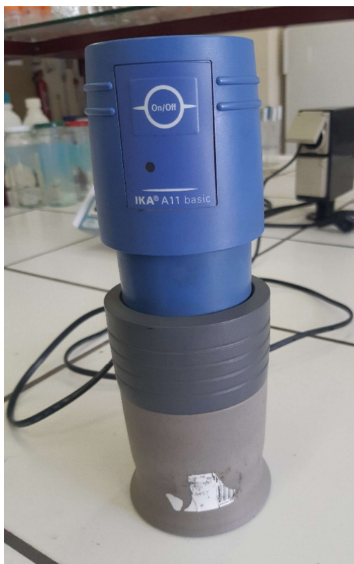
Figure 39: Basic analytic mill used for milling the waste and CEBs samples.
