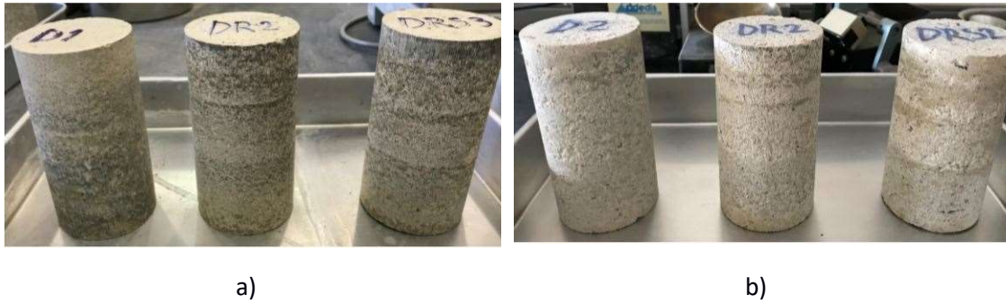
Figure 16: Specimens submitted to cycles of accelerated aging: a) before; b) after [46].
