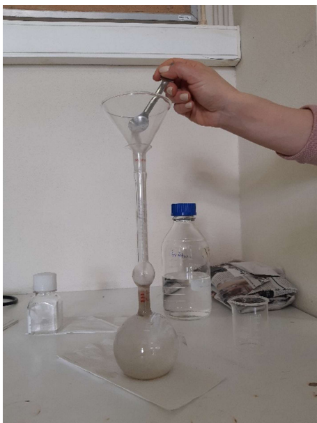
c) Mass being added to the flask;
