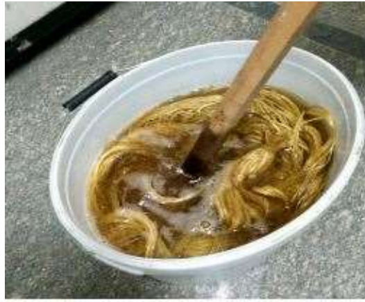
Figure 14: Banana fibres under chemically treatment to be incorporated on CEBs [36].
