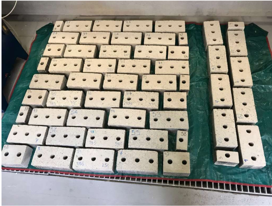
Figure 33: Blocks during the cure process in humid chamber.
