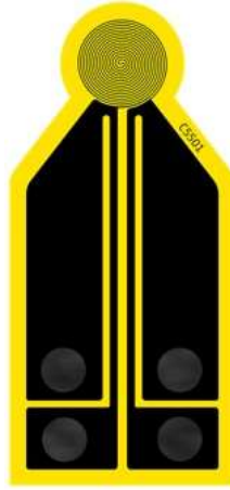
Figure 42: Kapton-insulated sensor used on TPS analyses [81].
