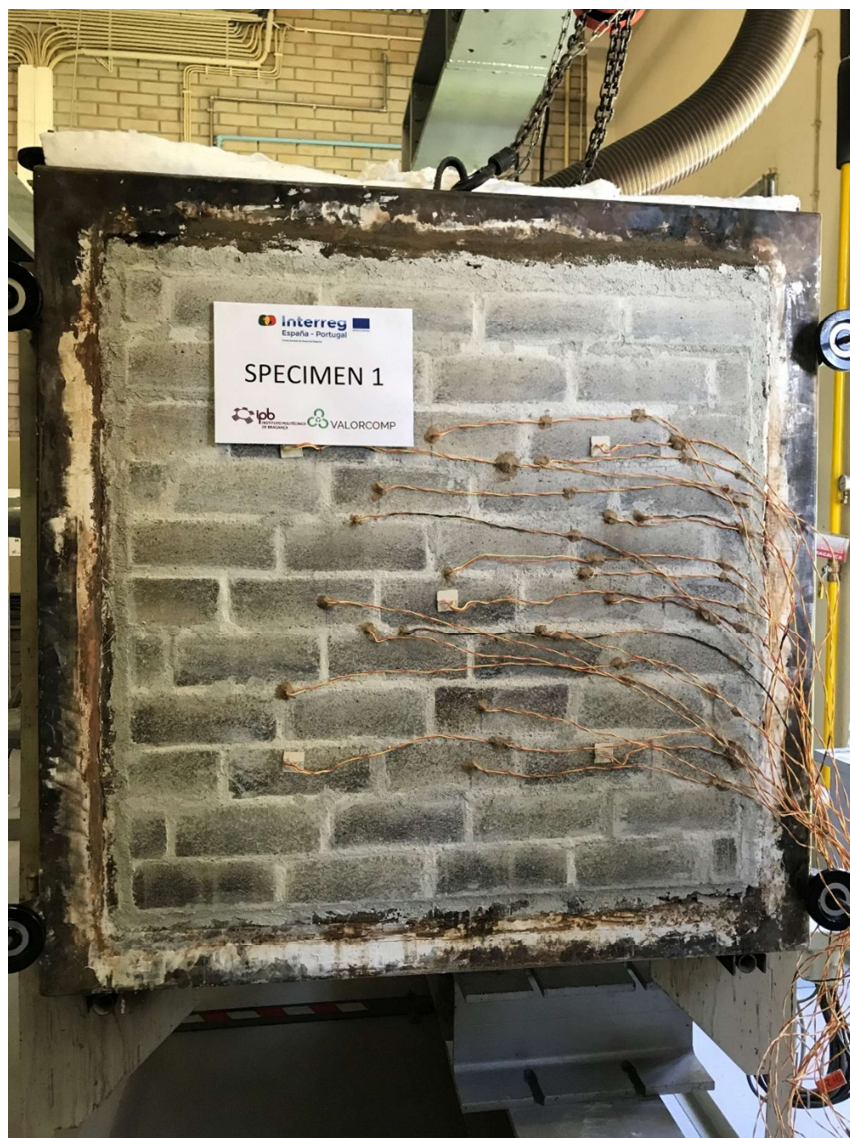
Figure 51: View of the instrumentalized panel from its unexposed surface.
