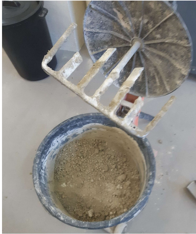
Figure 31: Materials prepared to be mixed in a mortar mixer.
