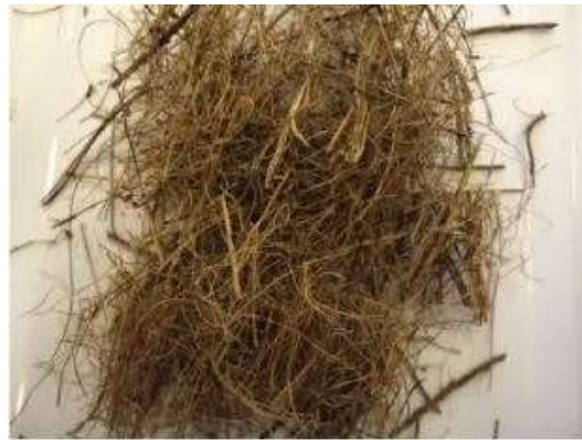
Figure 13: Cut Date-Palm fibres to be incorporated on the CEBs [35].
