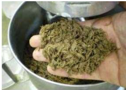
Figure 12: Krafterra fibres to be incorporated in the CEBS [32].
