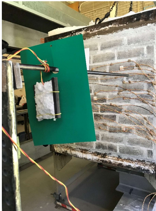
Figure 54: Thermocouple installed to monitor the ambient temperature at the laboratory during fire test.
