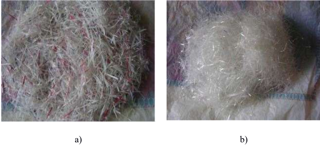
Figure 15: Plastic fibres to be incorporated on CEBs: a) from carry bags [40]; b) from plastic bottles [40].
