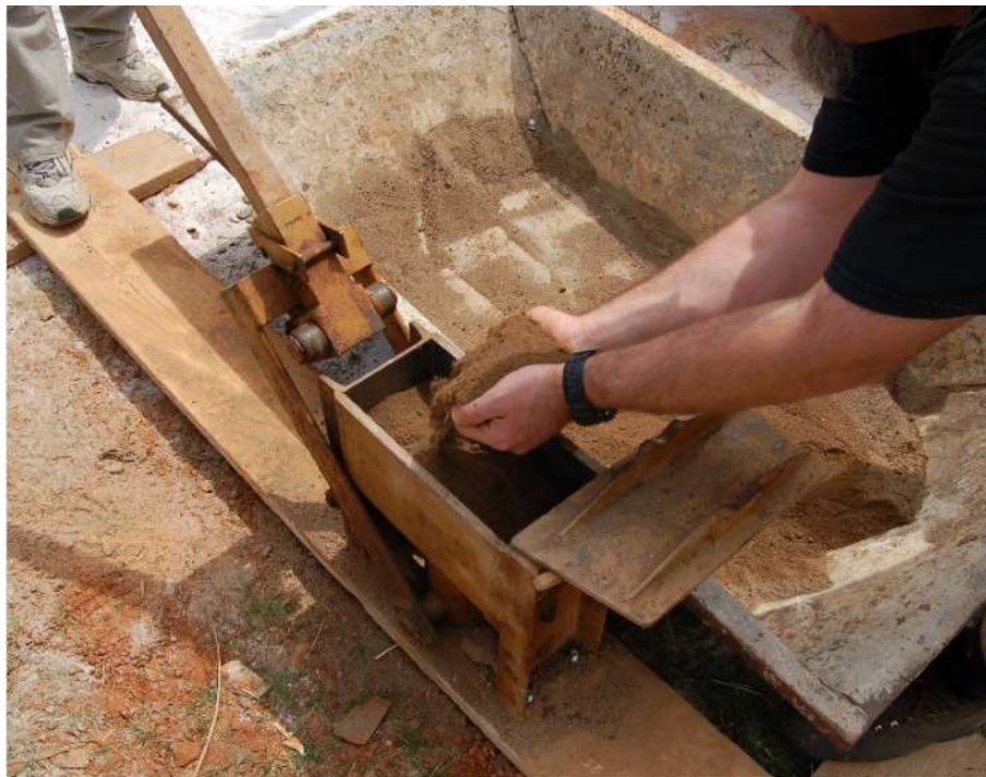
Figure 9: Example of a CEB CINVA-Ram press machine [23].
