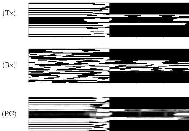
Figure 3: Quantized spectrograms of preambles for IEEE 802.11n: transmitted spectrogram (Tx), received spectrogram (Rx) (with 0 dB SNR) and the spectrogram reconstructed (RC) using the CDAE neural network. The black regions on the left represent parts of the spectrogram not used in the learning process, on account of their apparent lack of distinctive visual content (compare with Figure 2).
